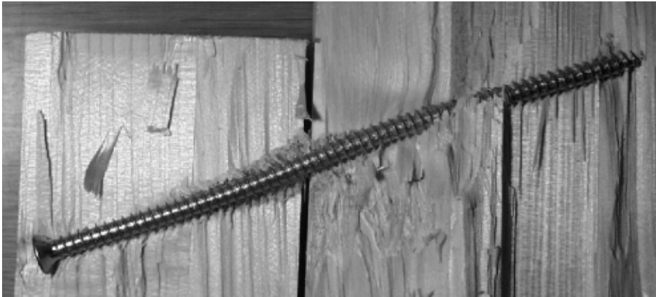
Figure 4: Sliced specimen with self-tapping screw
