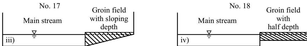
Figure 5.22. Schematic side view in streamwise direction of the experiments No. 17 and 18 where the dead-zone volume is reduced by 50% compared to the reference case.
