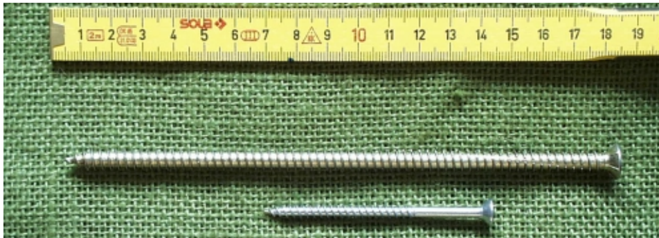
Figure 1: Screws used for reinforcement
