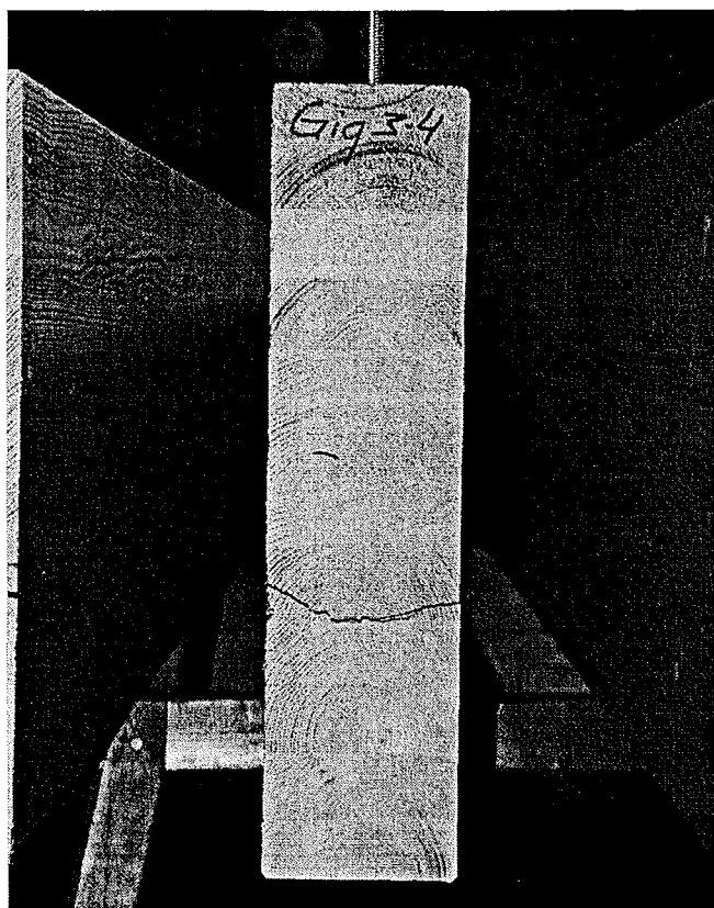
Figure 17: Tensile failure perpendicular to the grain
