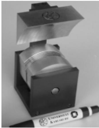
Figure 6.19: The entire offset cylindrical parabolic reflector antenna for the 76.5 GHz ACC radar.
