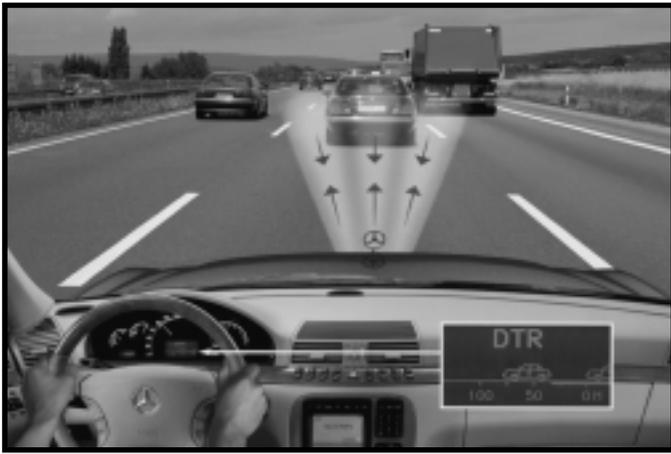
Figure 1.1: An ACC radar system at 76-77 GHz in Mercedes Benz S-Class models.
