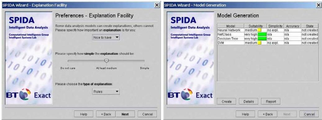
Figure 2: Choosing preferences in the Wizard. Left: the dialog for an explanation facility of methods. Right: ranking of data analysis methods according to user preferences before model creation
