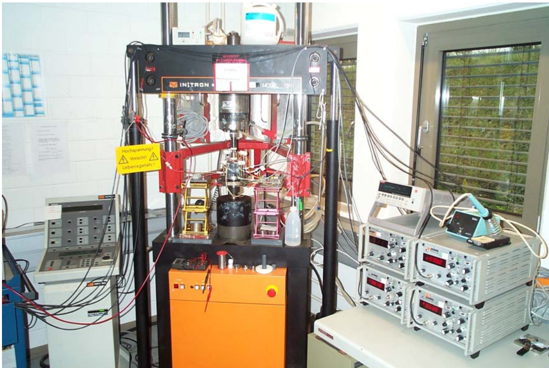
Figure 2.3.4. Photographs of the experimental set-up for combined electromechanical tests. (up) test fixture consisted of a polymer container, a spherical joint and alumina disks; (down) a part of the total experimental system with Instron machine, electrometer and four strain amplifiers.
