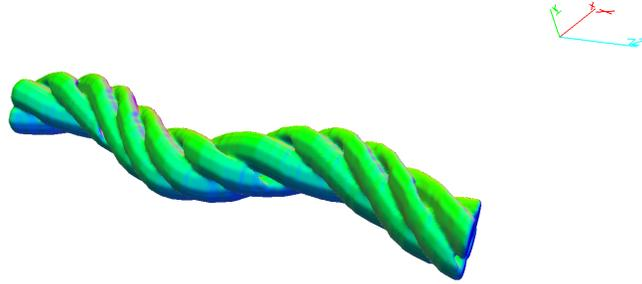
Figure 6: Twisted deck structure fiber.
