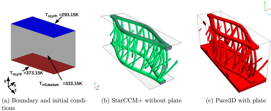
Figure 7: Boundary conditions and simulation environment (LC1).
