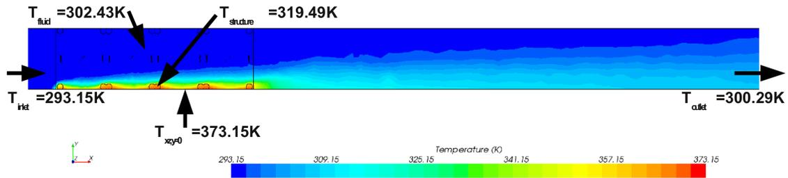
Figure 10: Temperature distribution in the  $xy$ -layer (LC2).
