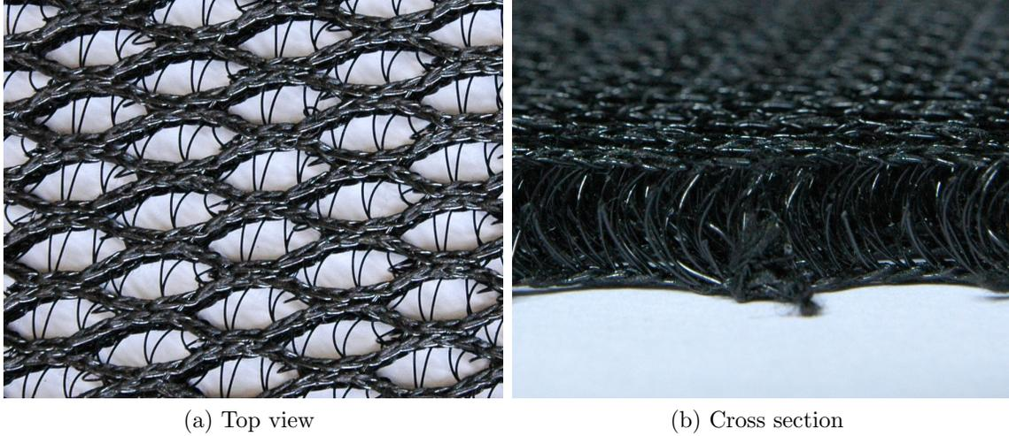
Figure 3: Textile spacer fabrics at high resolution.
