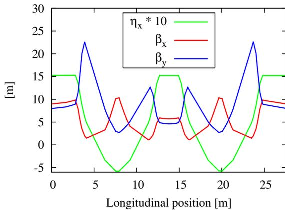
Figure 5: Low- $\alpha_c$ -optics with a momentum compaction factor of  $2 \cdot 10^{-5}$ , an RMS bunch length of 0.60 mm (2.0 ps), a natural emittance of 280 nm rad, tune values of  $\nu_{x,y} = (6.45, 2.96)$  and chromaticity values of  $\nu'_{x,y} = (-8.84, -8.31)$ .
