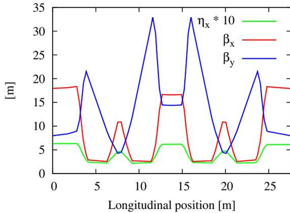
Figure 2: Low-emittance optics with a natural emittance of 38.3 nm rad, tune values of  $\nu_{x,y} = (7.13, 1.67)$  and chromaticity values of  $\nu'_{x,y} = (-15.90, -7.16)$ . One super period of the ANKA lattice is shown.
