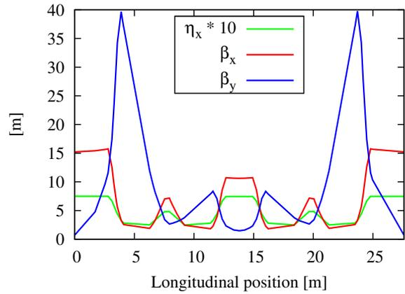
Figure 3: Low- $\beta_y$  optics with a vertical beta of 0.7 m in the straight sections, an emittance of 51 nm rad, tune values of  $\nu_{x,y} = (6.44, 4.53)$ , and chromaticity values of  $\nu'_{x,y} = (-11.10, -12.69)$ .
