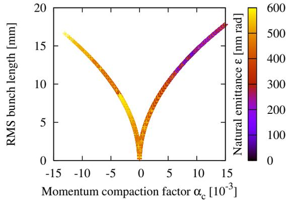
Figure 4: Relationship between momentum compaction factor  $\alpha_c$ , natural emittance, and natural RMS bunch length for an infinitesimal current at 2.5 GeV as calculated by the GLASS method.
