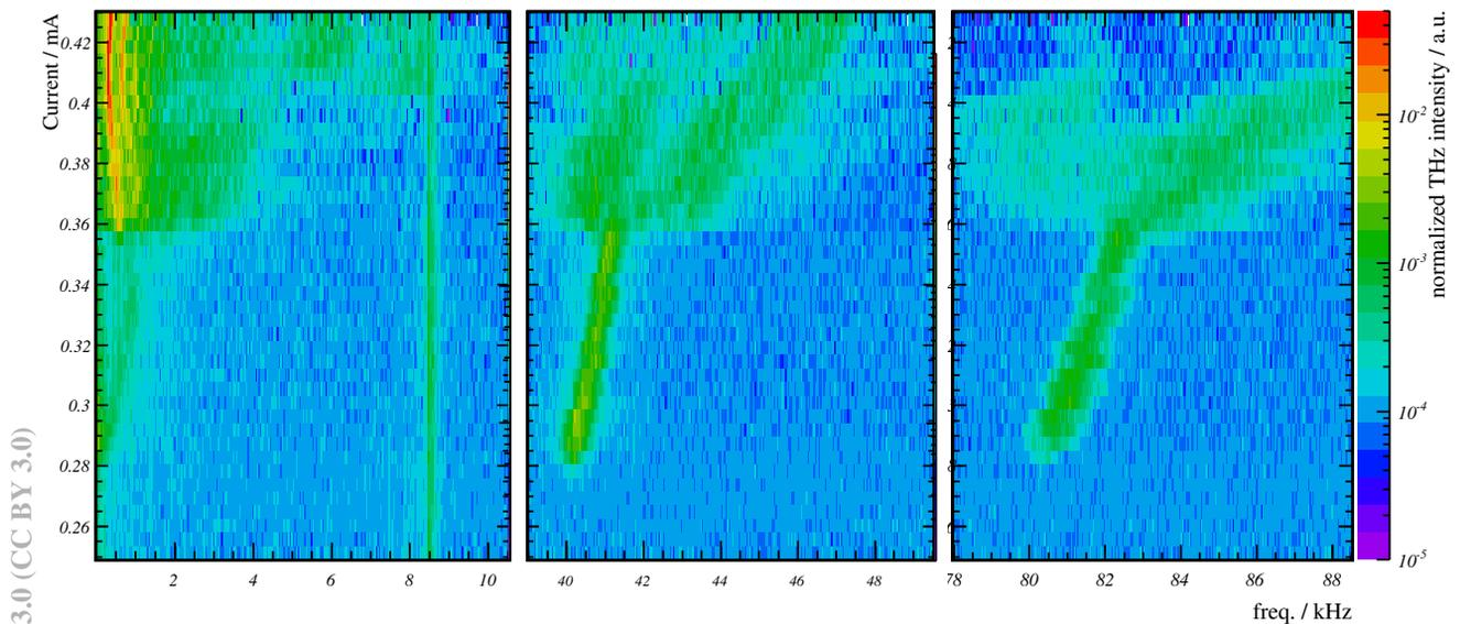
Figure 1: Instability spectrum of low frequency bursting is shown on the left diagram. Bursting occurs at currents  $> 0.28$  mA and changes mode at  $0.36$  mA. The main instability can be found at about  $400\text{--}600$  Hz and drifts with the current. Its harmonics are also clearly observable. The  $1f_s$  frequency line can be seen at  $8.5$  kHz. The middle and left figure show typical bursting patterns with onset at the same thresholds.
