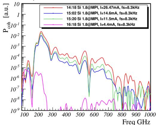
Figure 4: Spectra of CSR for different currents at the synchrotron frequency of 8.3 kHz. As expected there are additional high frequency components above the bursting threshold that disappear for low currents.
