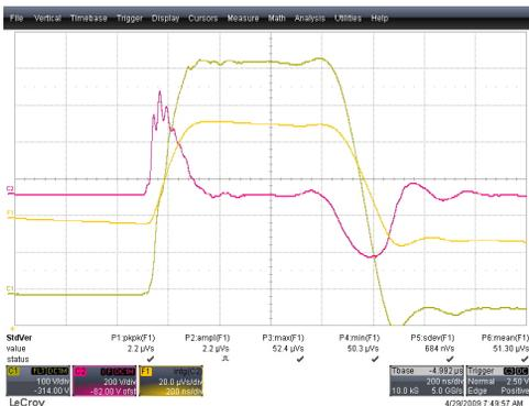
Figure 3: Current pulse for the BO extraction kicker (green), induced voltage on the coil (pink) and integrated field (yellow).
