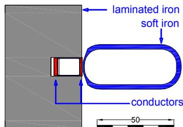
Figure 1: Cross section of SR injection septum.
