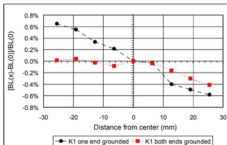
Figure 4: Transverse field homogeneity of integrated field.
