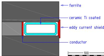
Figure 2: Cross section of Storage Ring injection kicker.
