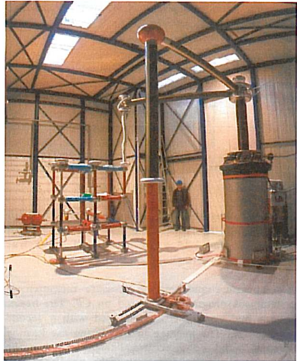
Figure 1 Test facility "FATELINI 2" in the Cryogenic High Voltage Lab of KIT-ITEP with cryostat and cryogenic bushing (right side), high voltage divider (foreground, middle), Marx generator (left) and high voltage transformer (background, far left).
