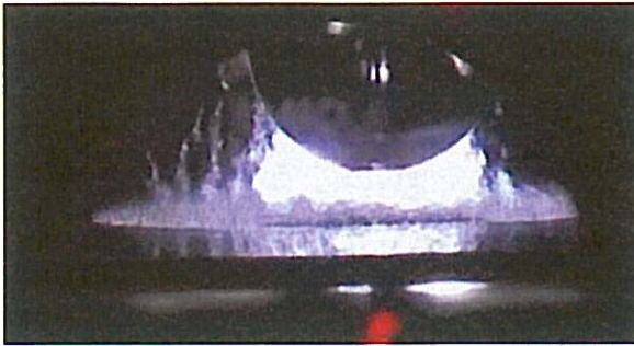
Figure 9 Sphere to plane arrangement at 0.3 MPa at the moment of maximum bubble generation. The amount of gas is considerably lower compared to the situation at lower pressure stages.
