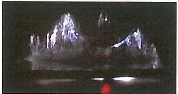
Figure 7 Sphere to plane arrangement at 0.2 MPa during strong bubble generation period.
