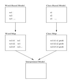
Figure 1. Class Hierarchy of language models within JRTk to implement a POS/word-based interpolated language model object.
