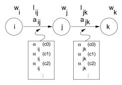
The lattice is traversed in an  $A^*$  like fashion. That means, for each edge  $e_{0i}$  originating from the start node, we compute the normalized forward probabilities  $\alpha_{0i}(c_l)$  and the log likelihoods  $l_{0i}$  as
