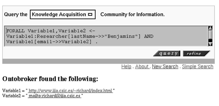
Fig. 9.2. Text-based Query Interface for Ontobroker
