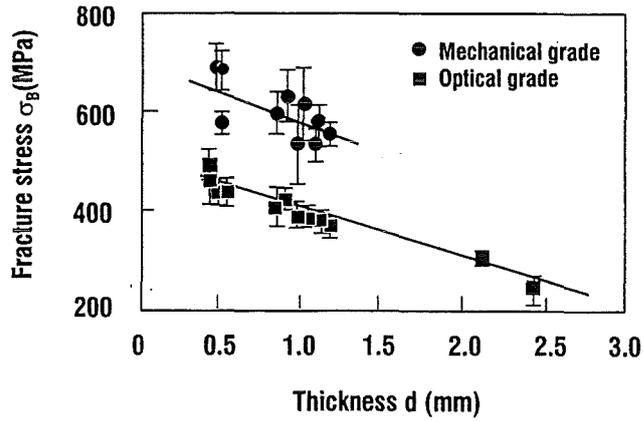
Fig. 29: Fracture strength of mechanical and optical CVD-diamond grades tested by DeBeers with growth surface under tensile stress [8].
