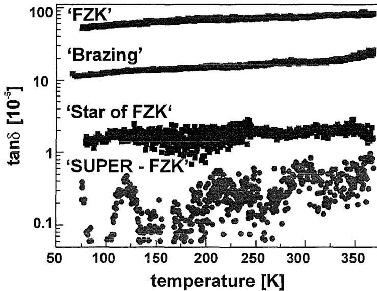
Fig. 19: Temperature dependence of  $\tan\delta$  at 145 GHz for the "FZK", "Brazing", "Star of FZK" and "Super-FZK" window disks.
