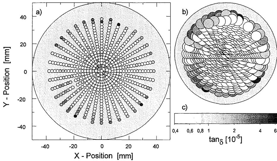
Fig. 22: Tan $\delta$  mapping for the "Super-FZK" window disk: a) demagnified spot size, b) actual spot size of 6mm and c) tan $\delta$  grey scale.
