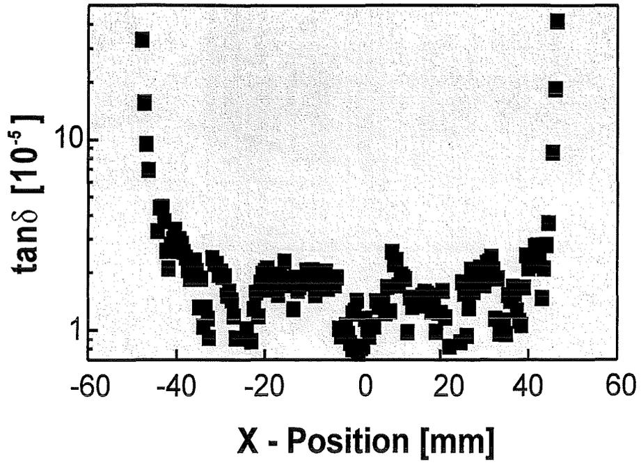
Fig. 23: Line scan across the diameter of the "Star of FZK" window disk.
