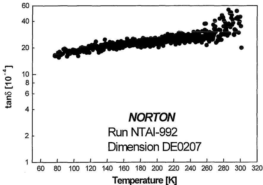
Fig. 27: Dielectric losses observed at 145 GHz in a CVD-diamond disk produced by the DC Arc Jet method.
