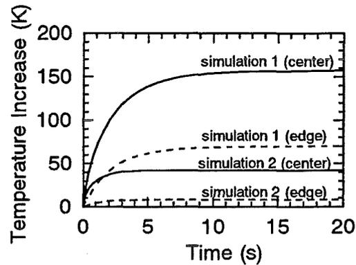
FIG. 7. Simulation results for two the types of window conditions. Simulation 1 shows the expected temperature increases vs time for the medium quality diamond disk at 0.5 MW, while simulation 2 shows those for the good quality disk at an rf power level of 1 MW.
