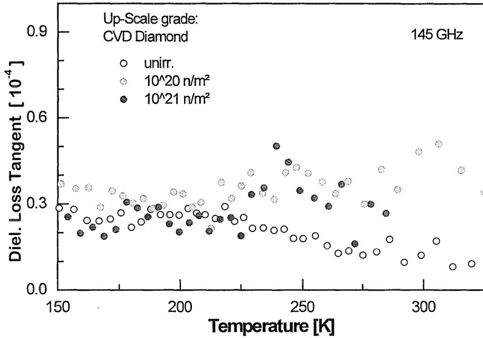
Fig.16a: The temperature dependence of dielectric losses observed at 145 GHz in the scale-up grade CVD diamond material before and after irradiation with fast neutrons.
