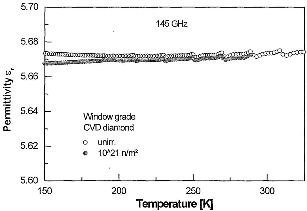
Fig.17b: The temperature dependence of the permittivity observed at 145 GHz in the window grade CVD diamond material before and after irradiation with fast neutrons.
