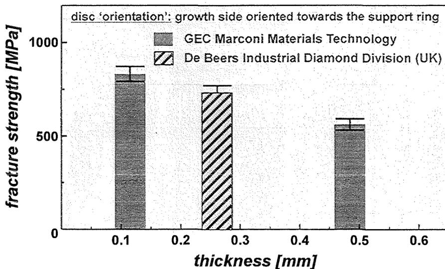
Fig. 28: The fracture strength of white (optical) CVD diamond grades tested with the growth side under tensile stress.
