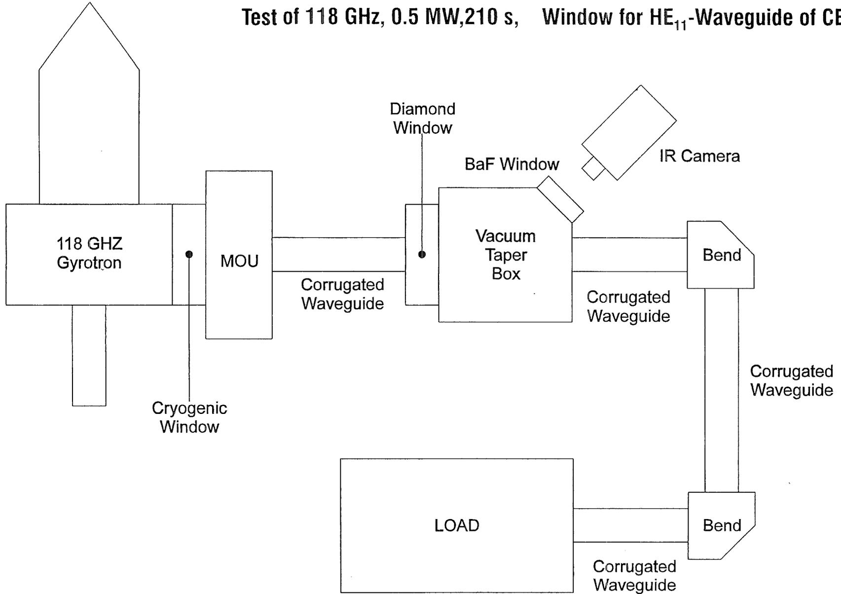
Fig. 11: Experimental arrangement for the test of the 118 GHz, 0.5 MW, 210 s CVD-diamond window in an evacuated HE<sub>11</sub>-waveguide at CEA Cadarache.
