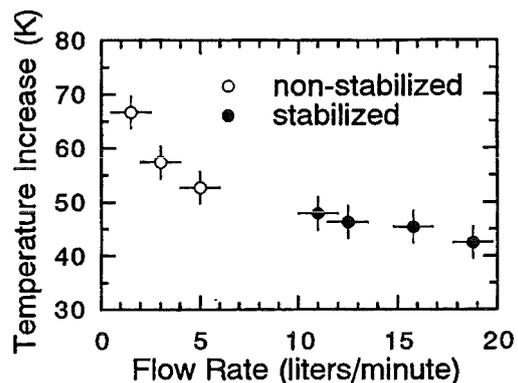
FIG. 5. Dependence of the window center temperature increase after 10 s (110 kW) operation on the flow rate of the cooling water. The closed circles represent stabilized temperature after 10 s, and the open circles represent nonstabilized temperature.
