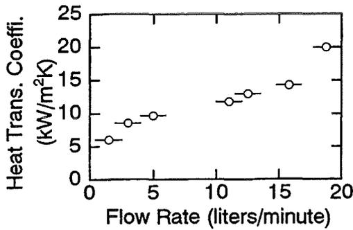
FIG. 6. Dependence of the heat transfer coefficient  $\alpha_c$  between the diamond edge and the cooling water on the water flow rate.  $\alpha_c$  is roughly proportional to flow rate.
