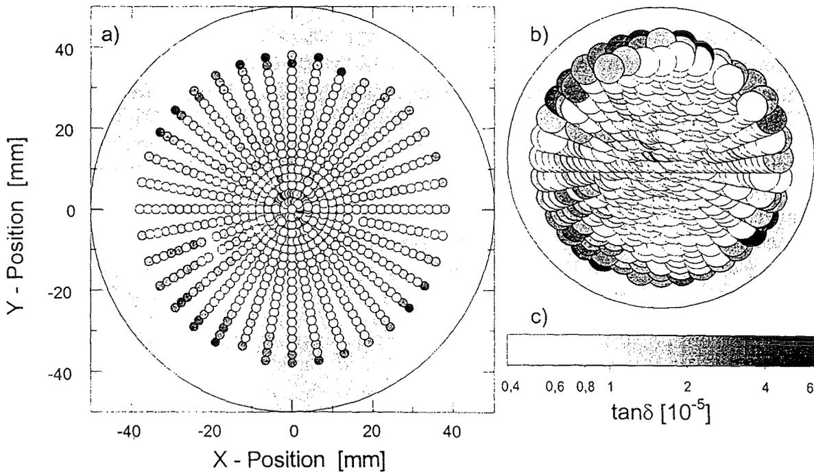
Fig. 6 a) Homogeneous 'Super-FZK' window (15DB1) with  $\tan\delta$  below  $10^{-5}$  in the central region; b) mapped with real spot size of 6mm and c)  $\tan\delta$  grey scale.
