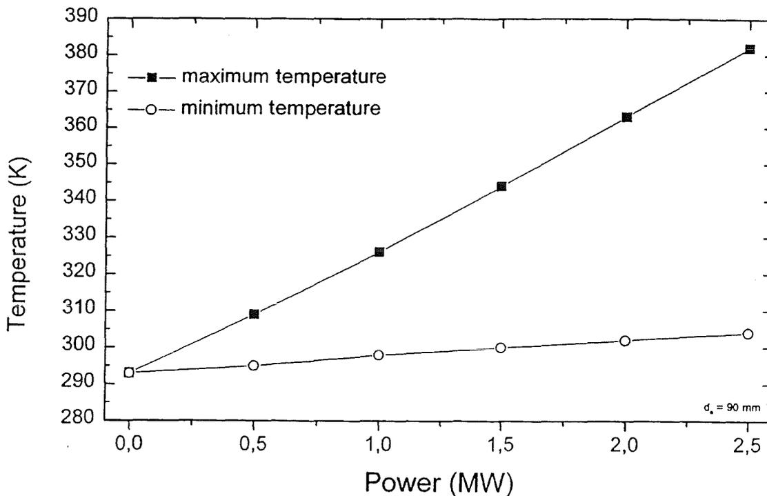
Fig. 7: Dependence of center and edge temperature of CVD-diamond window (outer disk diameter = 90 mm) on the transmitted mm-wave power (170 GHz).
