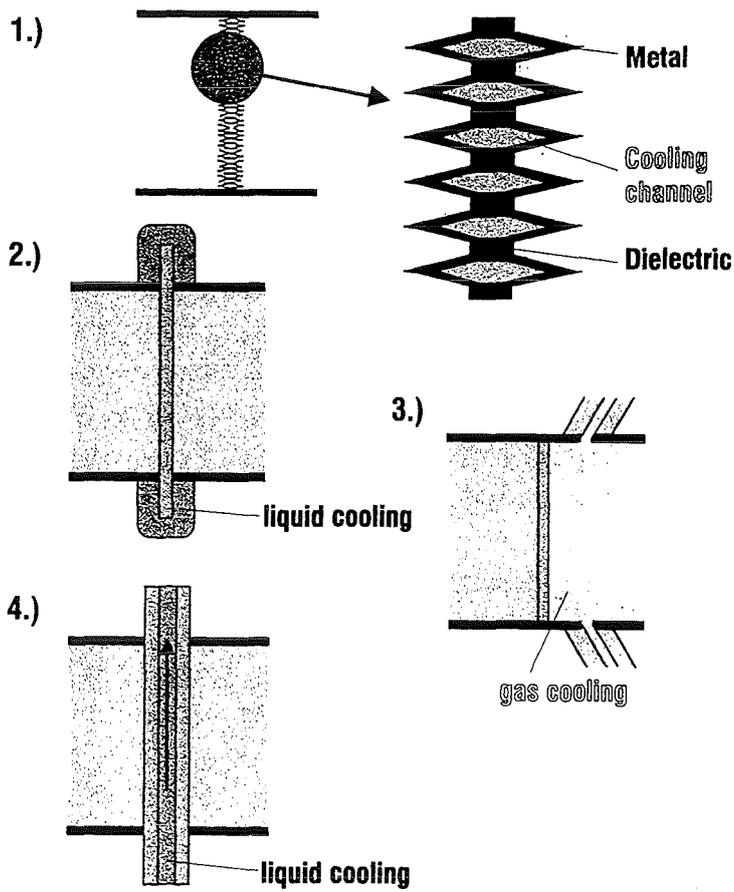
Fig. 2: General classes of high-power long-pulse capable microwave windows.
