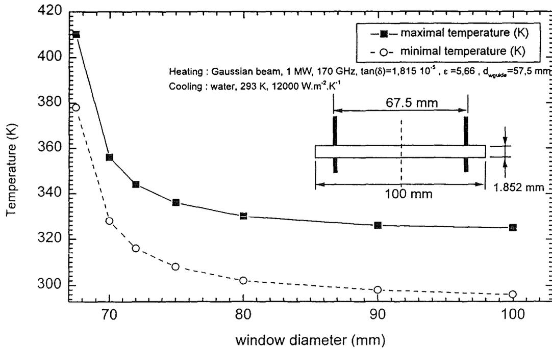
Fig. 5: Dependence of center and edge temperature of CVD-diamond windows on the width of the applied cooling rim at 1 MW mm-wave power (170 GHz).
