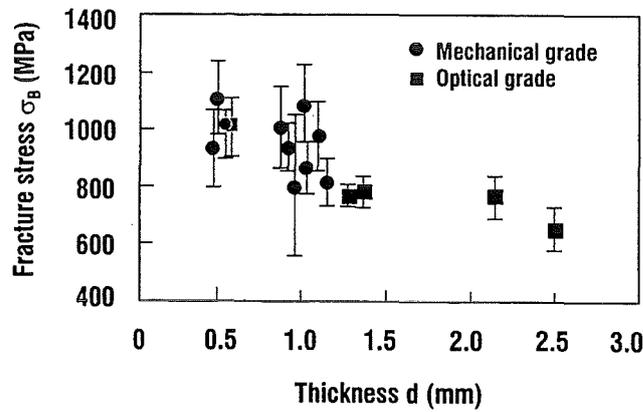
Fig. 30: Fracture strength of mechanical and optical CVD-diamond grades tested by DeBeers with nucleation surface under tensile stress [8].
