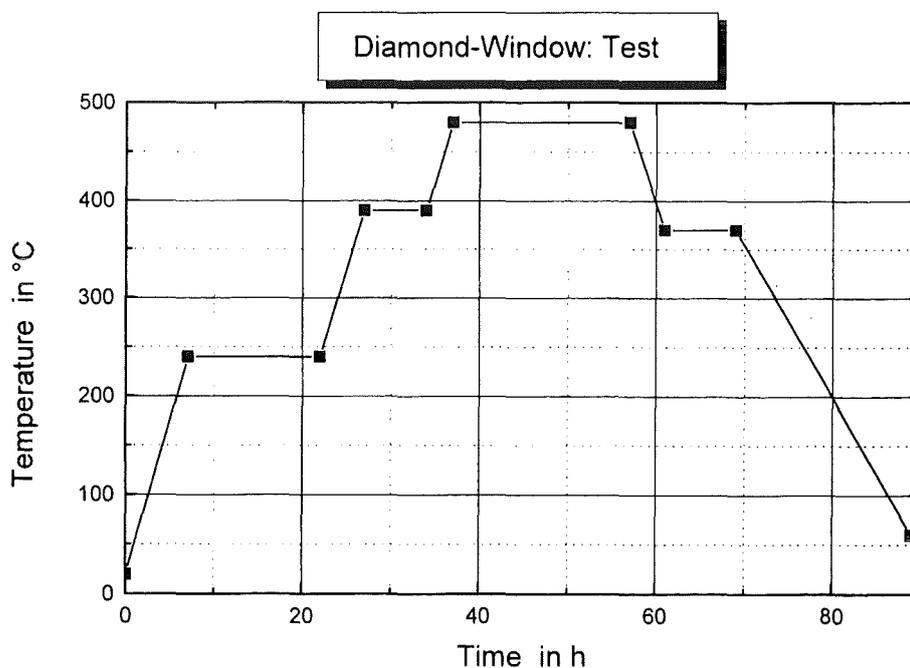
Fig. 3: Thermocycle applied to test diamond windows in a UHV vacuum oven.
