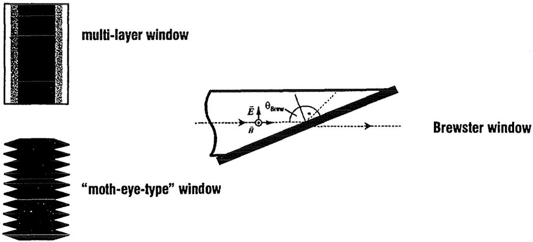
Fig. 1: Different solutions for broadband microwave windows.
