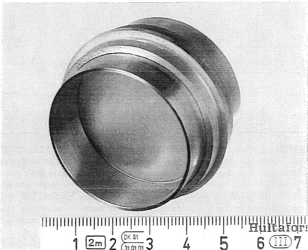
Fig. 4: Photograph of CVD-diamond bakeout test window unit.
