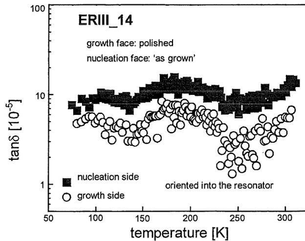
Fig. 25: Orientation dependent dielectric losses observed in CVD-diamond disk ERIII\_14.
