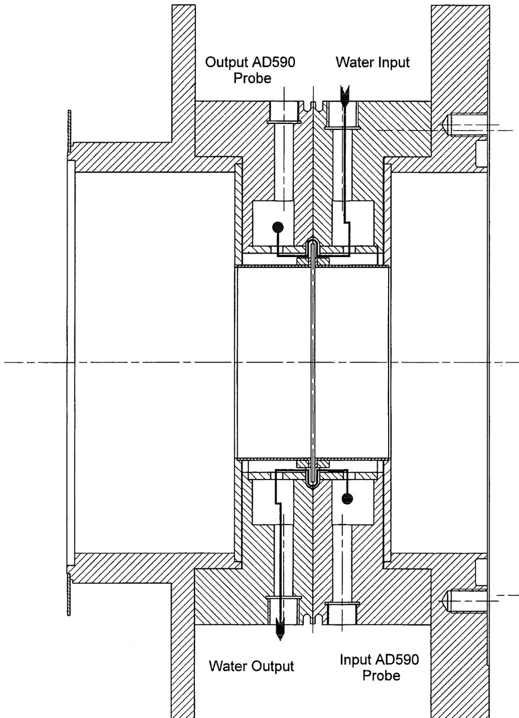
Fig. 5: Layout of the 118 GHz, 0.5 MW, 210 s CVD-diamond window.
