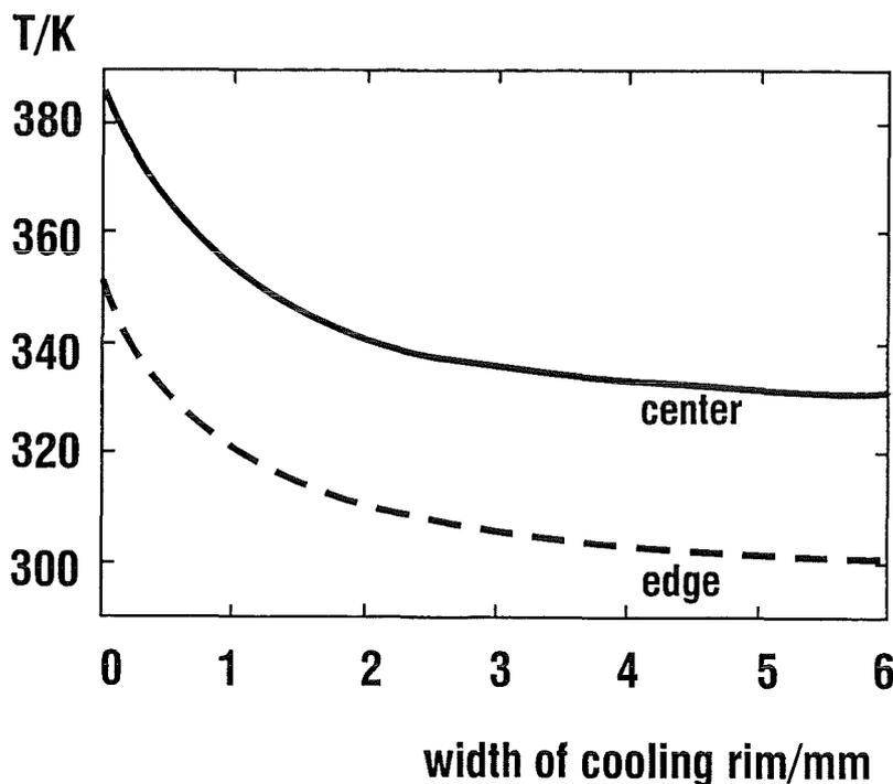
Fig.14: Dependence of center and edge temperatures of CVD-diamond window on the width of the applied cooling rim at 1 MW, 140 GHz.
