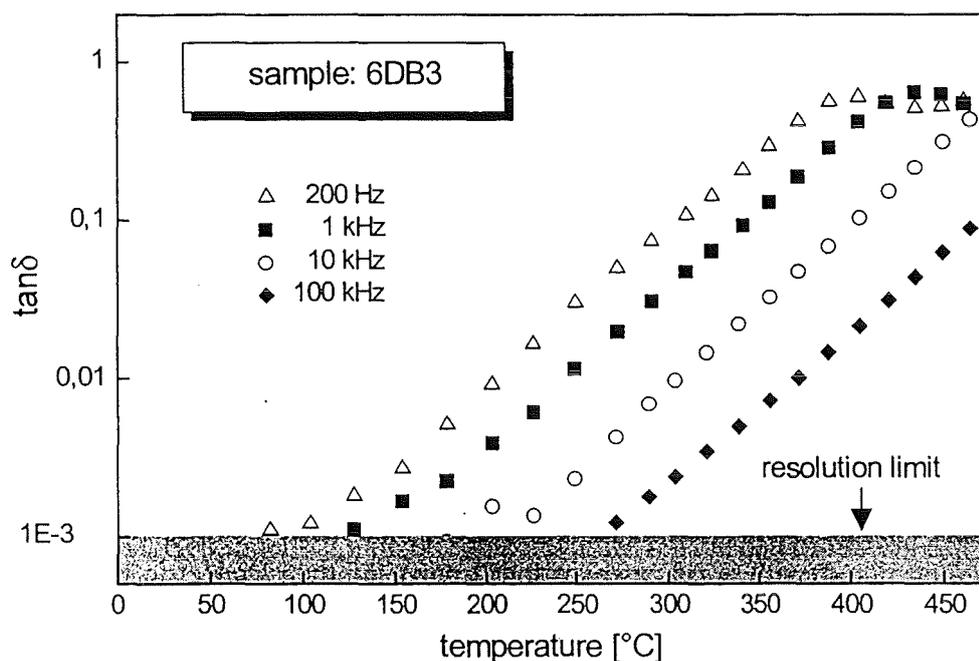
Fig. 1 Example for additional thermally excited losses.
