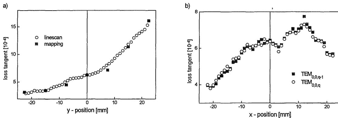
Fig. 18: Line scan of  $\tan\delta$  along the a) x-direction and b) y-direction in "FZK" disk at 145 GHz.
