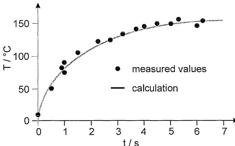
Fig. 12: Window center temperature increase versus time during transmission of a flattened rf beam at a frequency of 170 GHz and power level of 0.52 MW [1].
