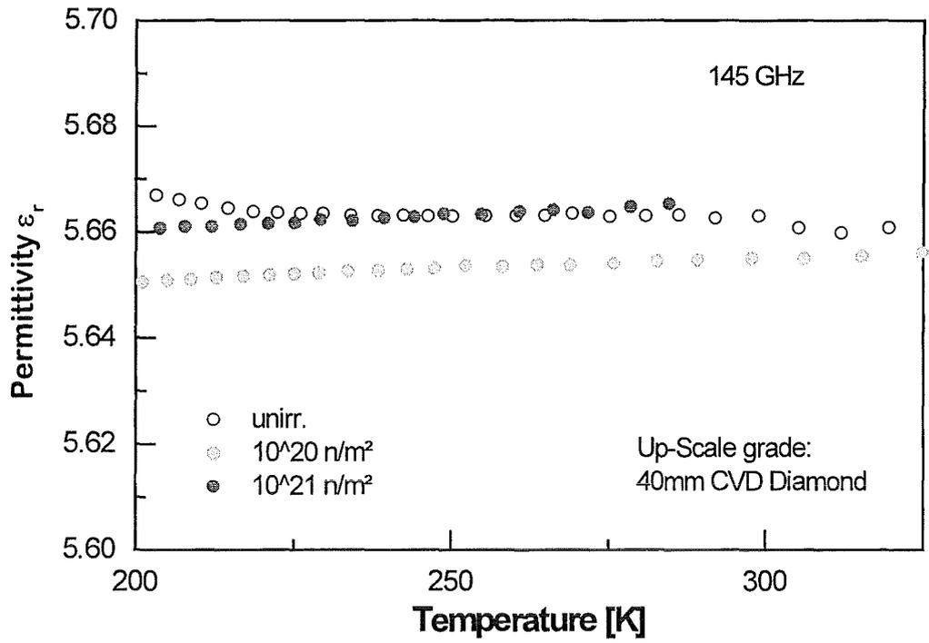
Fig. 17a: The temperature dependence of the permittivity observed at 145 GHz in the scale-up grade CVD diamond material before and after irradiation with fast neutrons.
