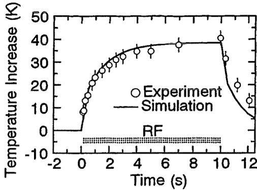
FIG. 4. Time behavior of the window center temperature increase for a 110 kW–10 s millimeter wave beam transmission. Open circles represent the experimental data and the solid curve shows the simulation result taking a heat transfer coefficient of 20 kW/(m<sup>2</sup> K) into account.
