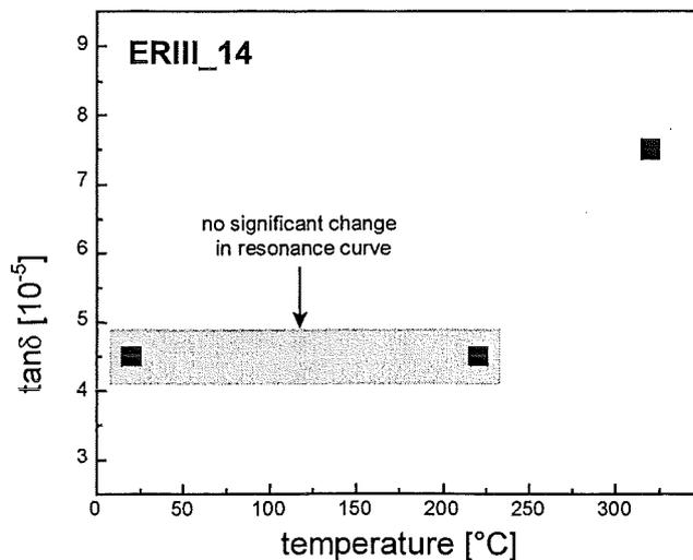
Fig. 26: Dielectric losses observed at 150 GHz and elevated temperatures in CVD-diamond disk ERIII\_14 (Annex 3).
