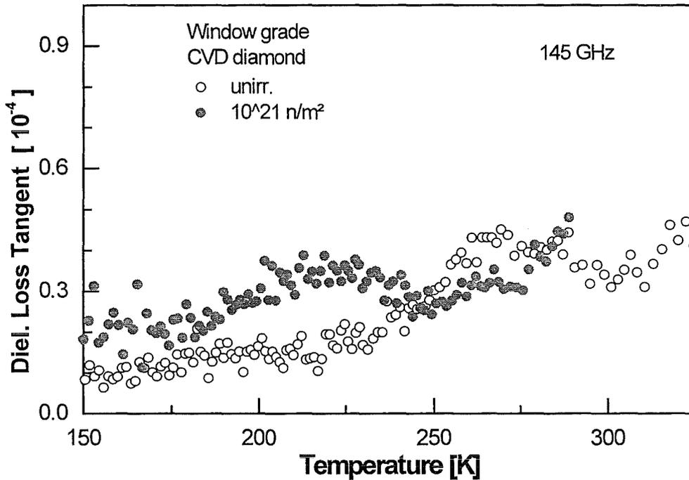
Fig.16b: The temperature dependence of dielectric losses observed at 145 GHz in the window grade CVD diamond material before and after irradiation with fast neutrons.
