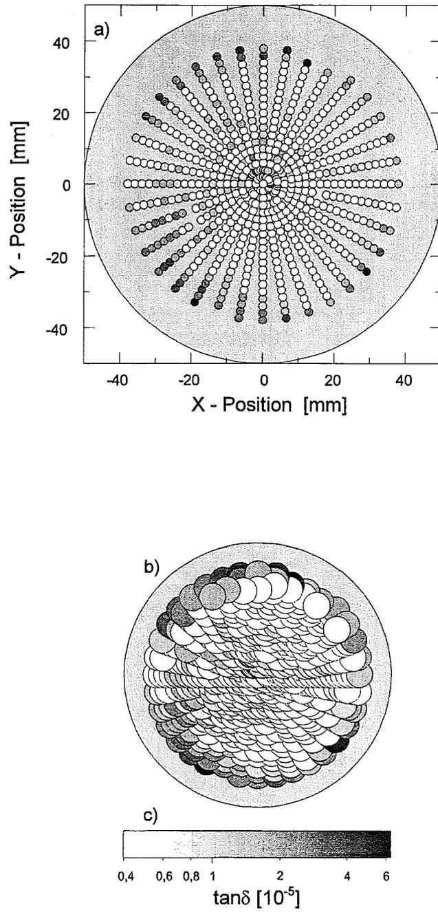
Fig. 9: Distribution of loss tangent values of the CVD-diamond window disk "Super-FZK".
