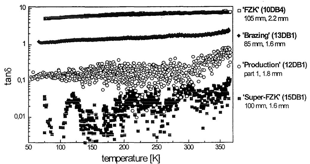
Fig. 2 Temperature dependence of CVD diamond windows from different grades (dimensions of disc given as diameter, thickness).
