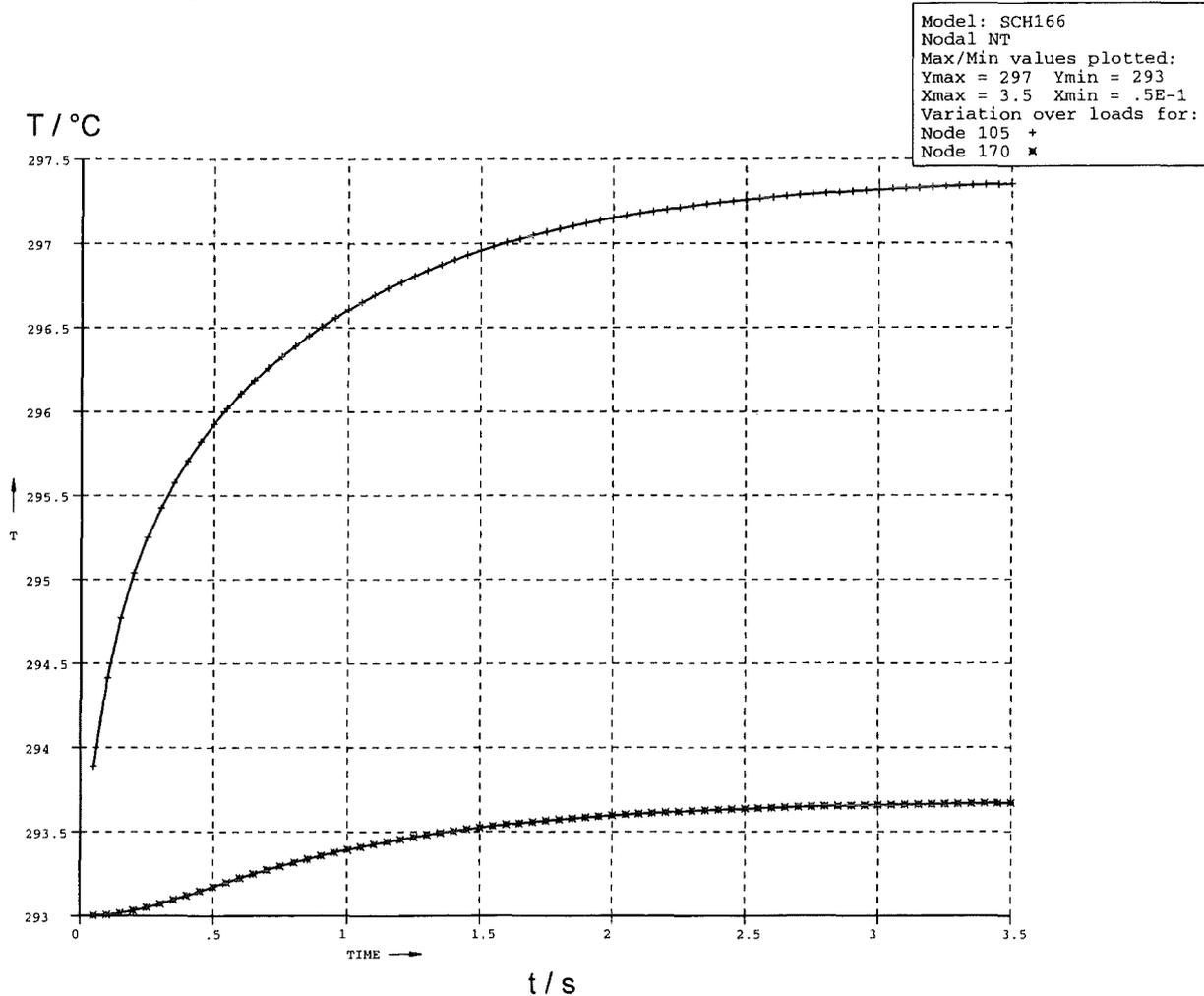
Fig. 10: Time dependence of center and edge temperatures of CVD-diamond window at 0.5 MW, 118 GHz (cooling water at 293 K).
