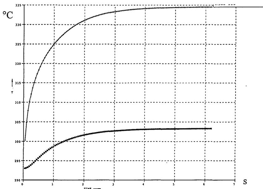
Fig. 15: Time dependence of center and edge temperatures of CVD diamond window at 1 MW, 140 GHz (width of cooling rim = 4 mm).
