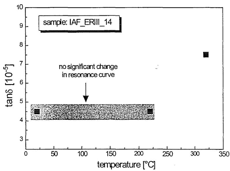
gyrotron window (below 100 °C in the centre of window) - an increased  $\tan\delta$  was observed.
