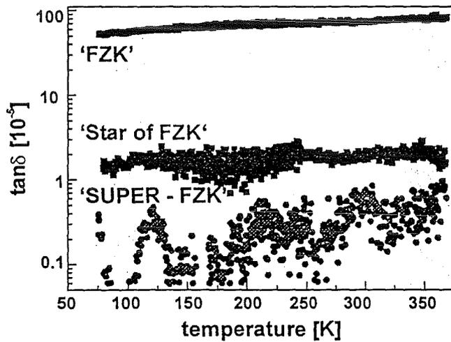
Fig. 1 Temperature dependence of  $\tan\delta$  at 145 GHz for the 'FZK', 'Star of FZK' and 'Super-FZK' window discs.
