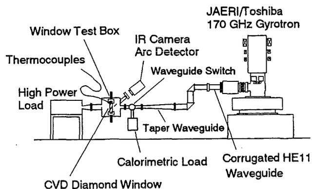
FIG. 3. Schematic drawing of the experimental setup using the JAERI gyrotron facilities (transmission power: 170 GHz, 110 kW, 10 s).
