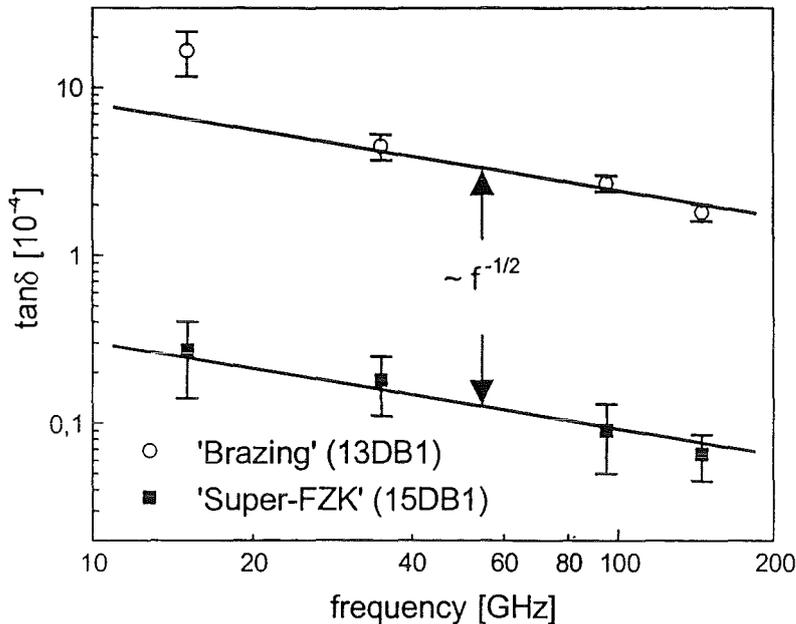
**Fig. 4** Frequency dependence of the locally inhomogeneous 'Brazing' - window (13DB1) and the homogeneous 'Super-FZK' - window (15DB1).
