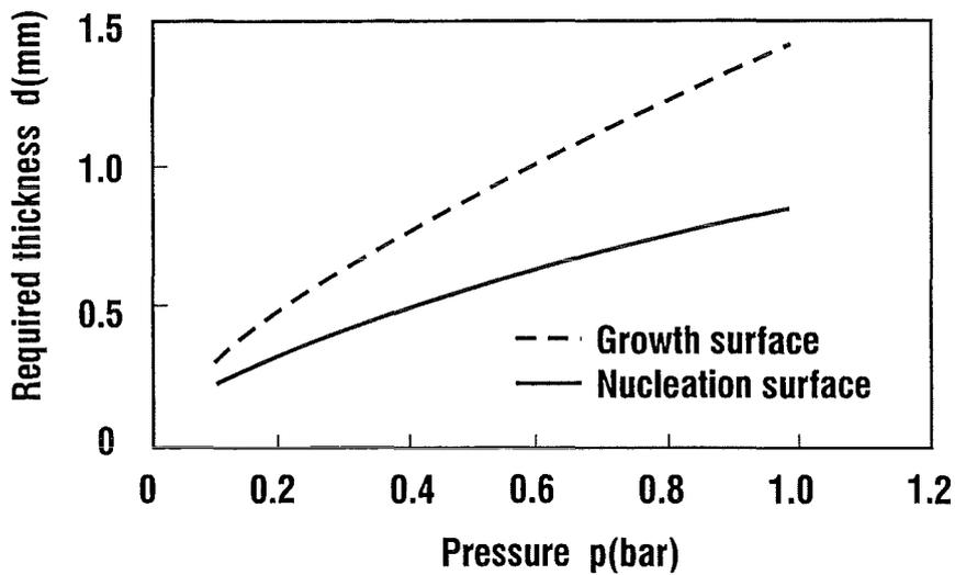
Fig. 31: Required minimum thickness of a CVD-diamond window with 80 mm aperture diameter and a safety factor of 4 in dependence of the pressure difference with growth or nucleation side under tensile stress respectively [8].
