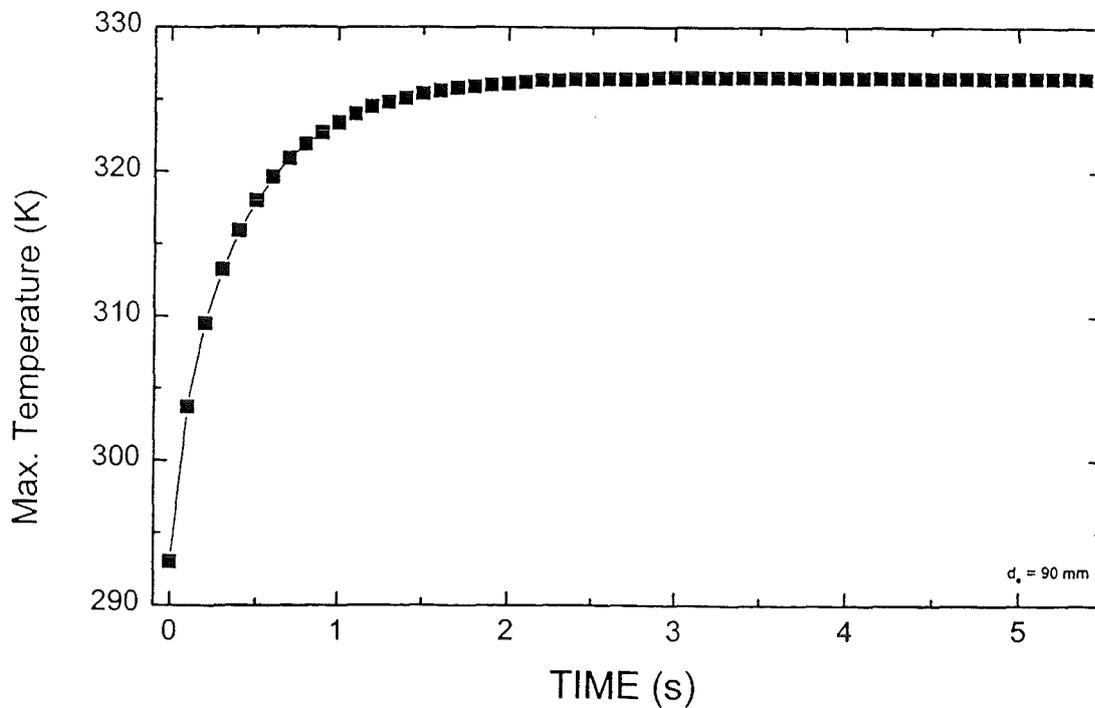
Fig. 6: Time dependence of center and edge temperature of CVD-diamond window (outer disk diameter = 90 mm) at 1 MW (170 GHz).
