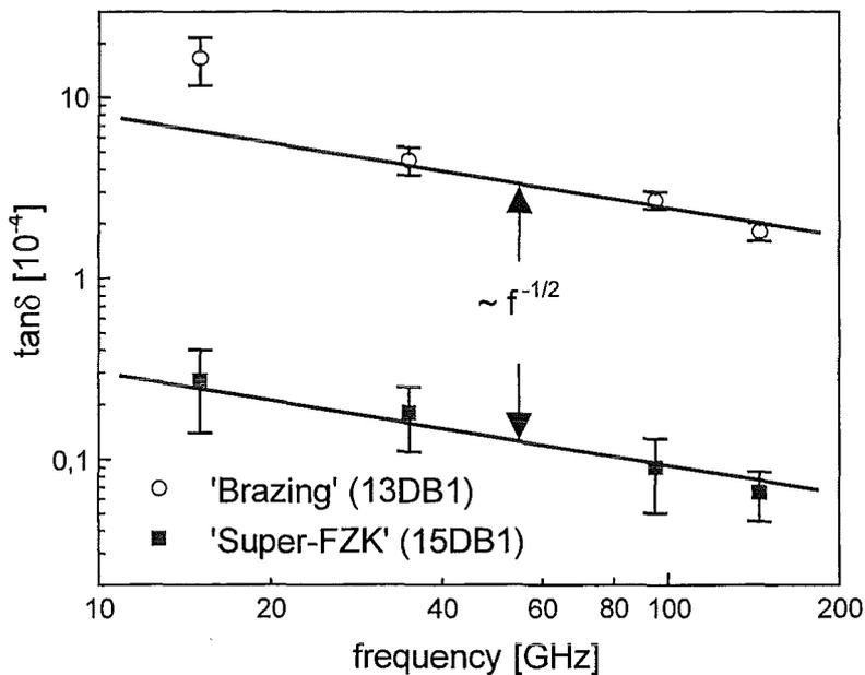
Fig. 20: Frequency dependence of  $\tan\delta$  of the locally inhomogeneous "Brazing"-window (13DB1) and the homogeneous "Super-FZK" - window (15DB1).
