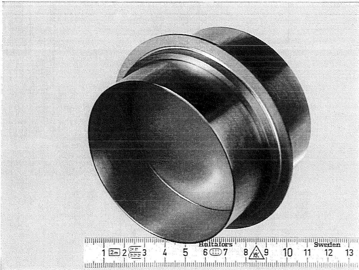
Fig. 7: Photograph of the CVD-diamond disk "Super-FZK" mounted to two Inconel 600 sleeves.
