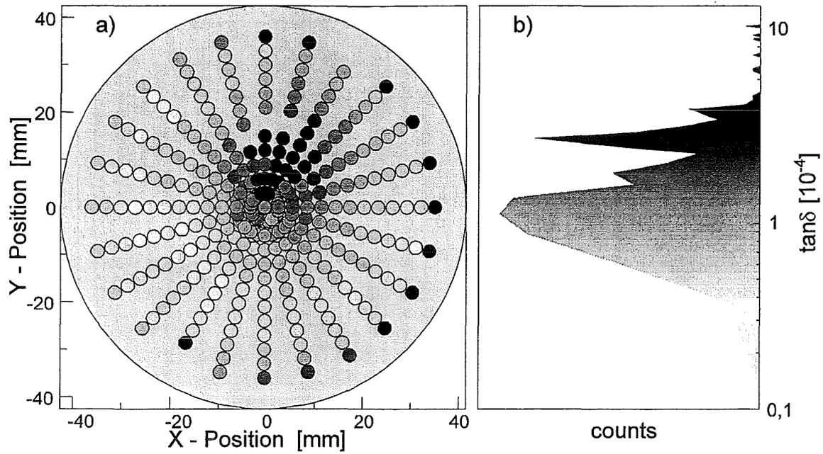
Fig. 21: Tan $\delta$  mapping for the "Brazing" window disk: a) demagnified spot size, b) distribution of measured tan $\delta$  points and their grey scale.
