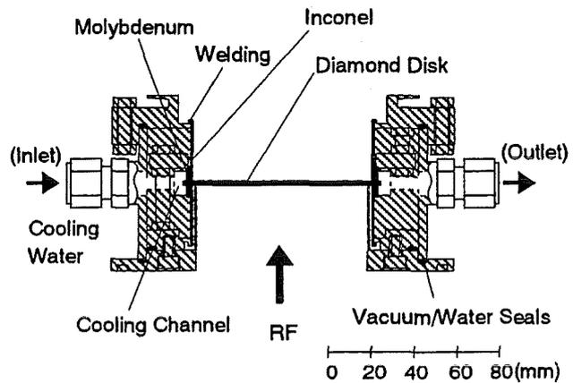
FIG. 2. Technical drawing of the cross section of the assembled diamond window.
