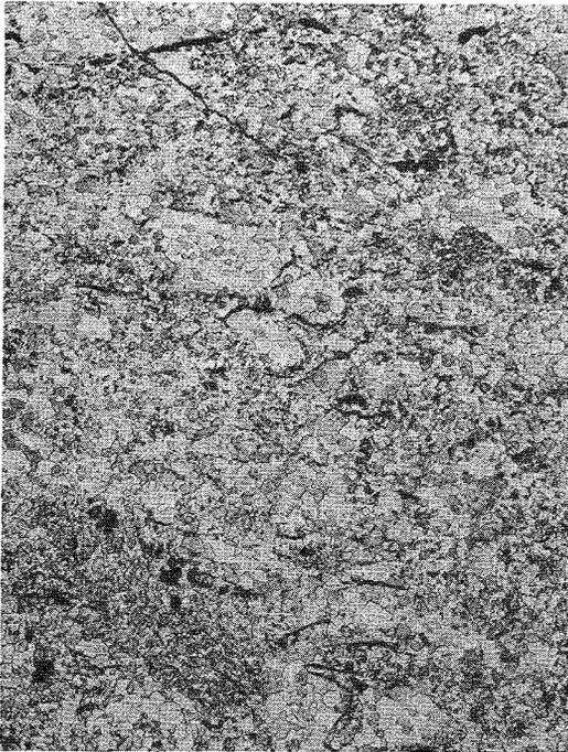
$\text{Th}_{0,05}\text{U}_{0,95}\text{O}_{2,21}$  (600°C, 24 h)
