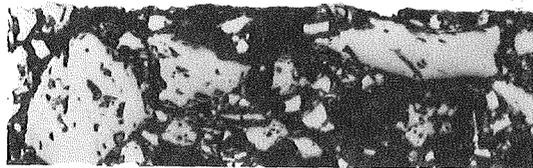
1.4988+(U<sub>0.7</sub>,Pu<sub>0.3</sub>)O<sub>1.97</sub>+Cs 800°C/1000 h
