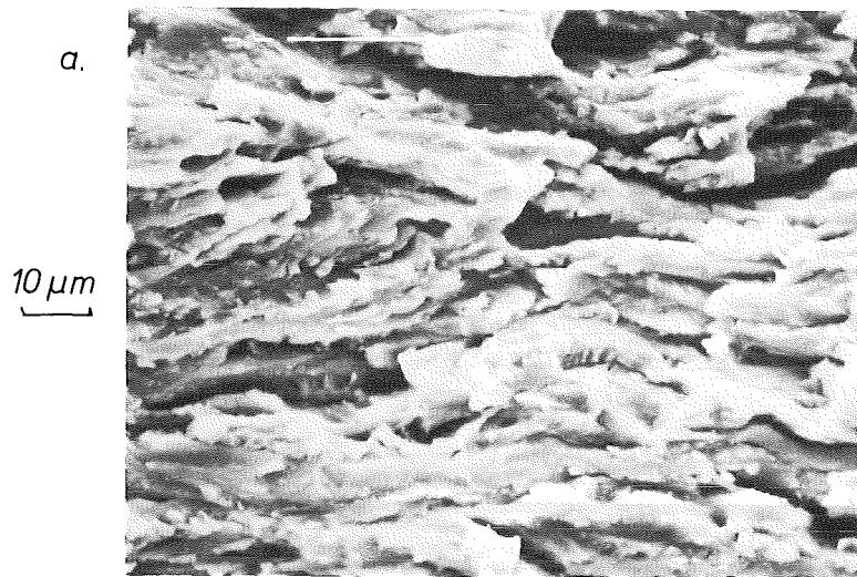
transgranular fracture surface
