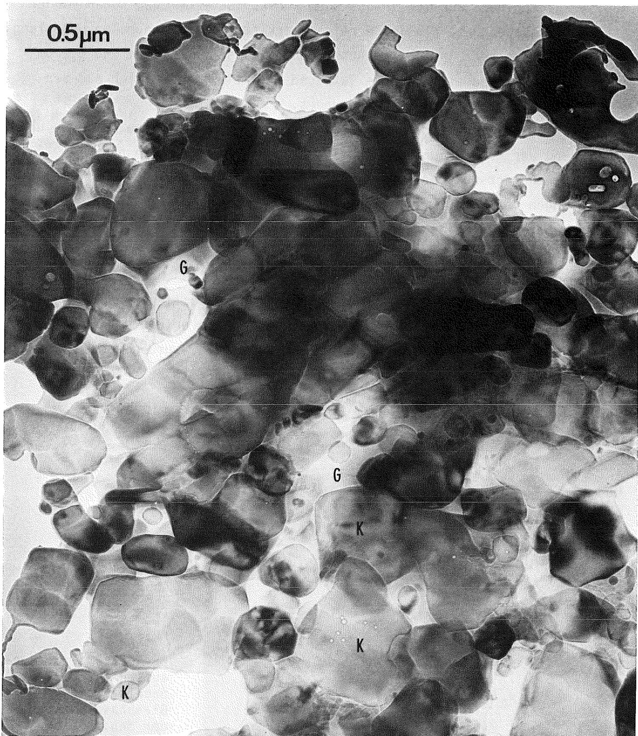
**Abb. 37: Probe HP 1** ( $T = 1050^{\circ}\text{C}$ ,  $p = 65 \text{ MPa}$ ).
