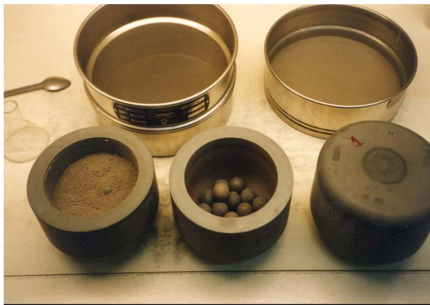
**Figure 4.6:** Ball mills and sieves
