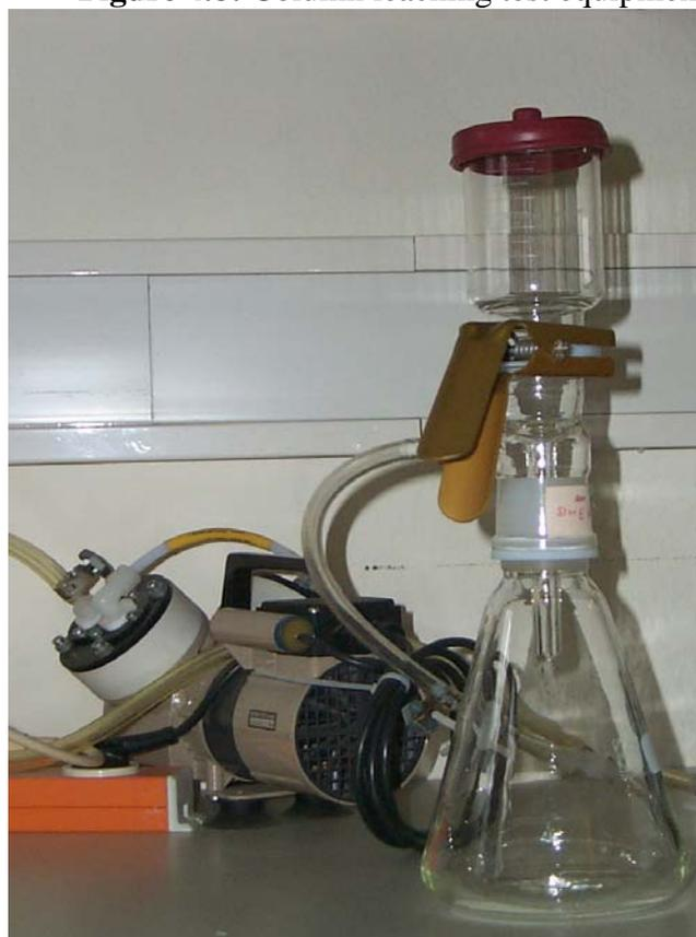
**Figure 4.9:** Vacuum filtration equipment
