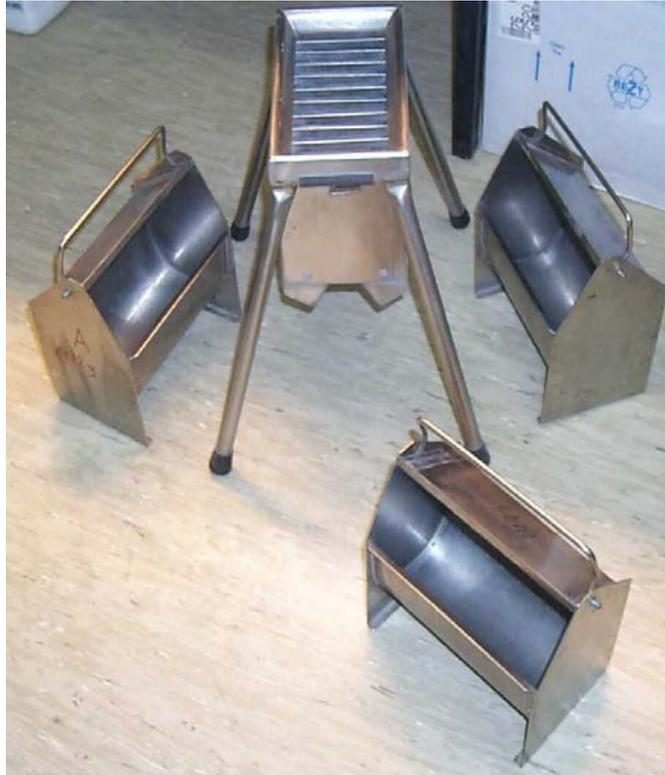
**Figure 4.5:** Riffle for sample subdivision
