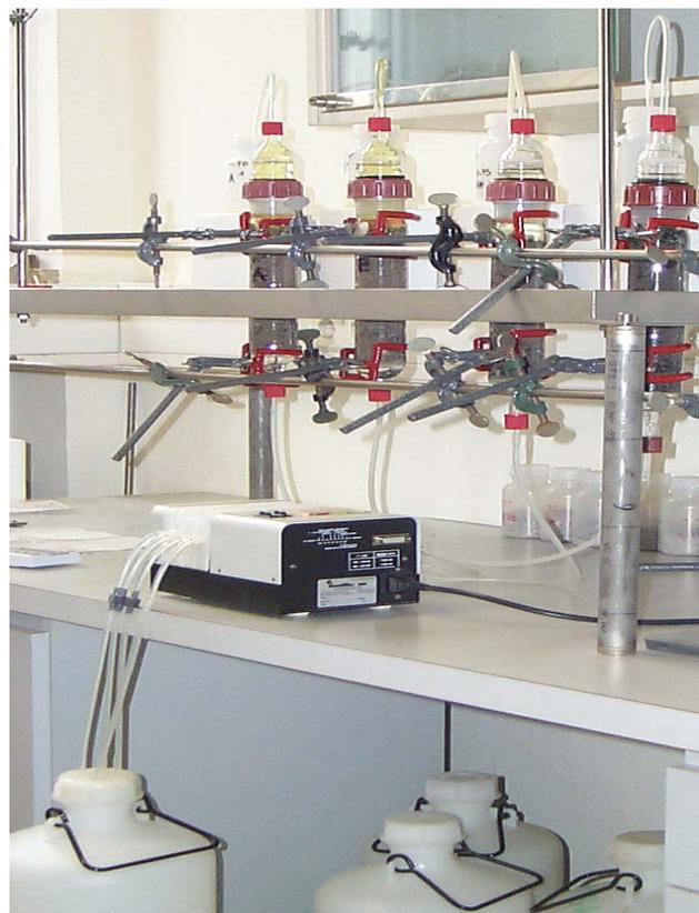
**Figure 4.8:** Column leaching test equipment
