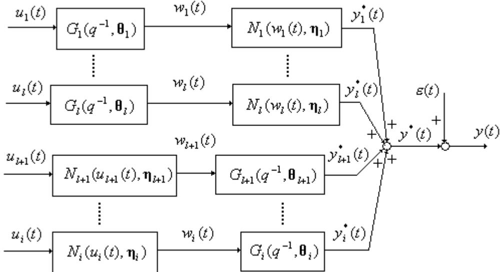
Fig. 3.11 MISO mixed Wiener and Hammerstein system
