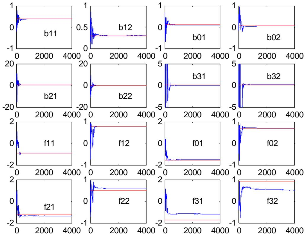
Fig. 6.6 The generalized Wiener system identification process with a N./S.=5% colored measurement noise
