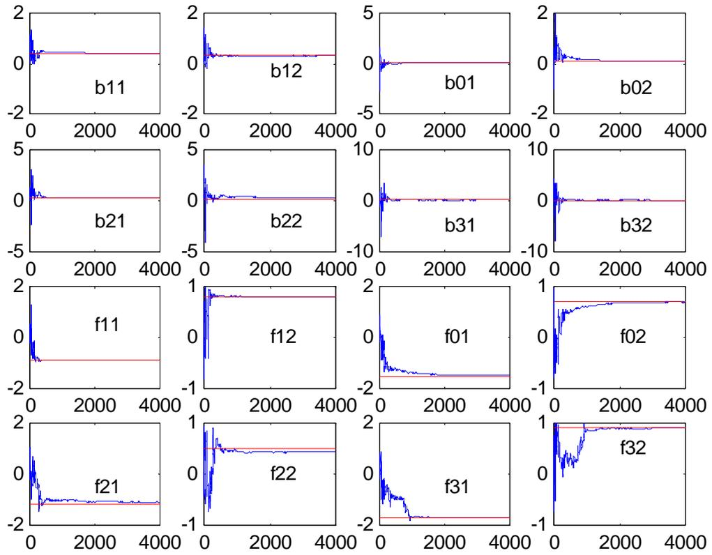
Fig. 6.5 The generalized Hammerstein system identification process with a N./S.=5% colored measurement noise
