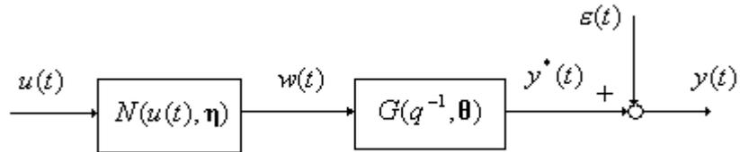
Fig. 3.2 Hammerstein system
