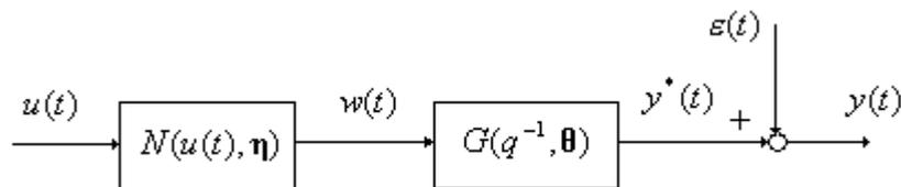
Fig. 1.3 Hammerstein system
