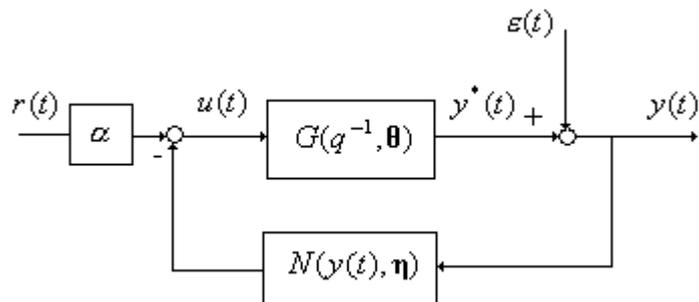
Fig. 3.4 Feedback-Hammerstein system
