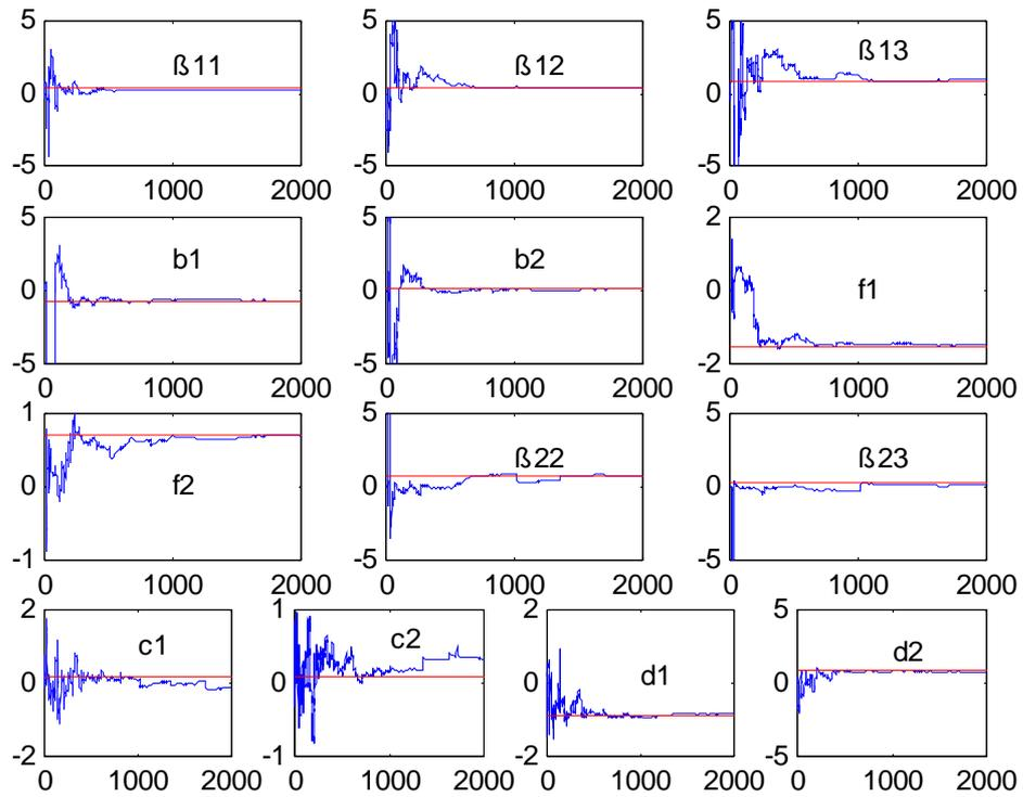
Fig. 5.6 Hammerstein-Wiener system identification process with two continuous nonlinearities with a N./S.=5% colored measurement noise
