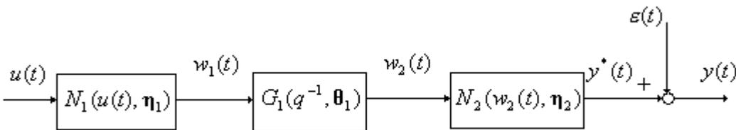
Fig. 5.2 Hammerstein-Wiener system (NLN)
