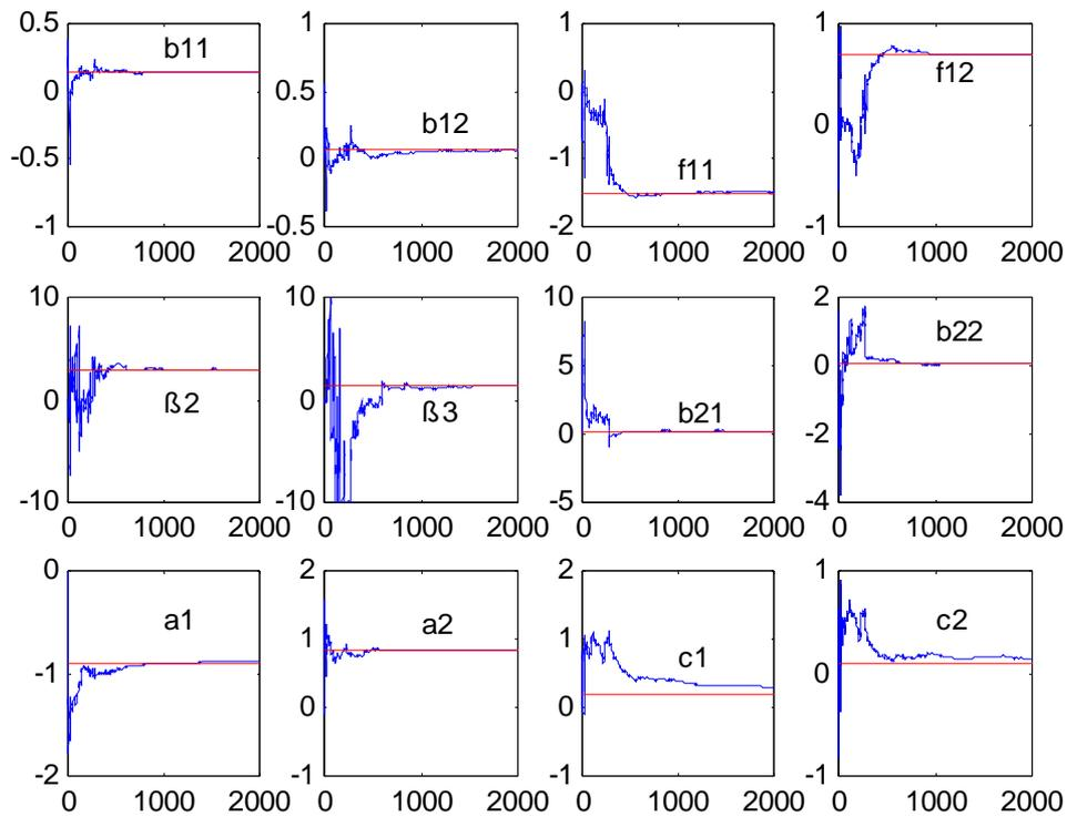
Fig. 5.4 The Wiener-Hammerstein system identification process with continuous nonlinearity with a N./S.=5% colored measurement noise
