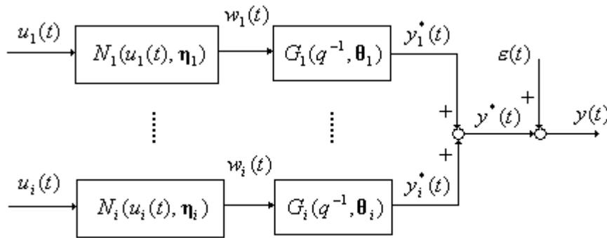
Fig. 3.10 MISO Hammerstein system
