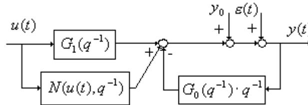
Fig. 6.2 Generalized Hammerstein system
