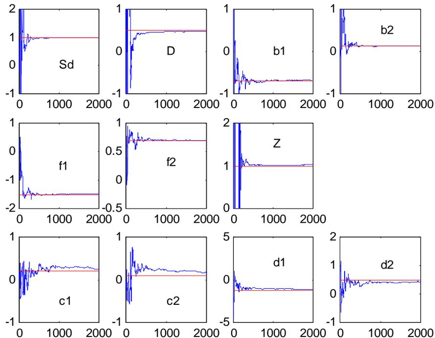
Fig. 5.7 Deadzone-Linear-Saturation system identification process with a N./S.=5% colored measurement noise
