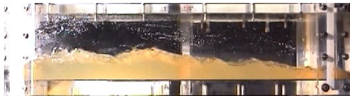
a) Partially reversed Flow. Large amplitude waves are present at the interface.
