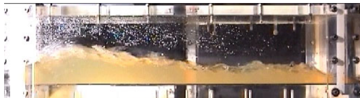
d) The volumetric flow rate of gas delivered by the blower is automatically reduced due to an increase in head losses.
