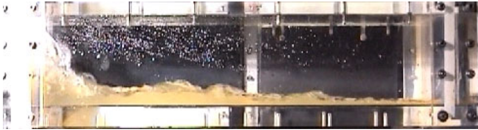
Partially reversed flow with imminent totally reversed flow.
