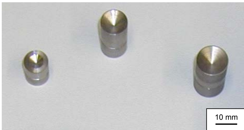
Fig. 2-2 Some tungsten Knudsen cells, fabricated by PLANSEE (Reutter, Austria).
