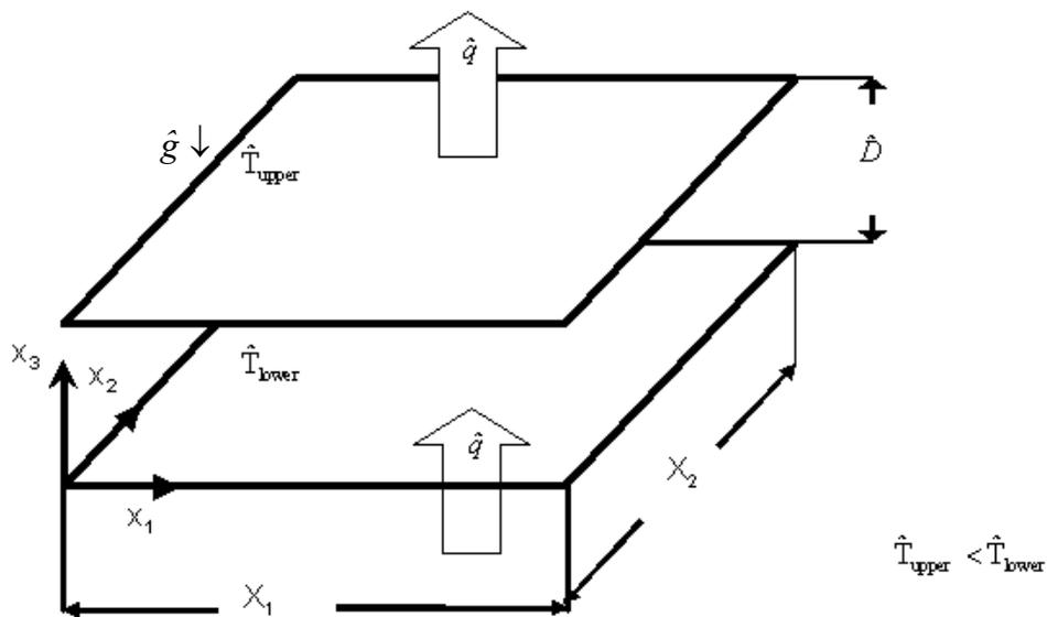
Fig. 3-2 Geometry as in TURBIT to describe Rayleigh-Bénard convection (RBC).
