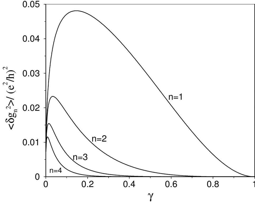
Figure 1.7: The ensemble-averaged amplitudes  $\langle \delta g_n^2 \rangle$  of the first four harmonics of mesoscopic Aharonov-Bohm oscillations. The coefficient is calculated for systems without spin-orbit interaction. For systems with strong spin-orbit interaction, the  $\langle \delta g_n^2 \rangle$  are reduced by an extra factor of  $1/4$ .
