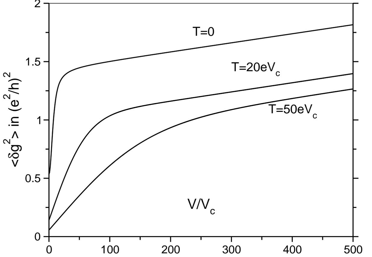
Figure 3.7: The voltage dependence of the conductance fluctuations as given by the interpolation formula (3.64), for the temperatures  $T = 20eV_c$  and  $T = 50eV_c$ . The  $T = 0$  result (see Figs. 3.5, 3.6) is also shown for comparison. It is clearly seen that only the offset (3.45), but not the slope of the asymptotic linear behaviour (3.53) is changed by the temperature, and the crossover towards the linear asymptotics is broadened on a voltage scale of the order of the temperature.
