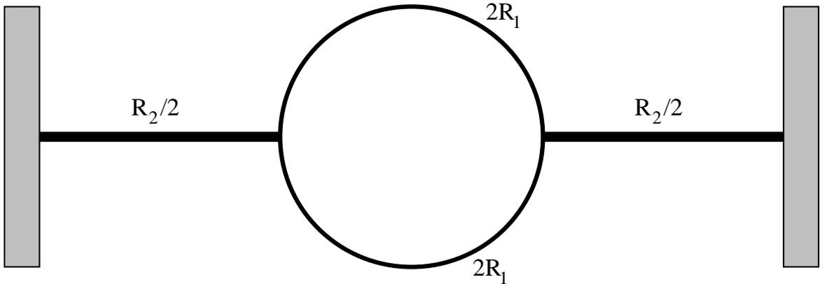
Figure 1.6: Two-terminal Aharonov-Bohm sample geometry which in the noninteracting limit shows the mesoscopic conductance oscillations (1.18). The geometrical coefficient  $\gamma$  is defined as  $\gamma = R_1/(R_1 + R_2)$ .
