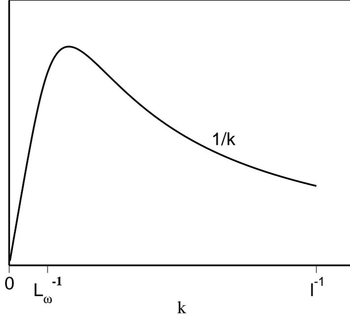
Figure 4.3: Plot of the absolute value of the integrand of Eq. (4.34) as a function of the gauge field momentum  $k$ . In the transverse gauge, the logarithmic contribution arises from the first term in brackets and is regularized at the lower limit by the other terms.
