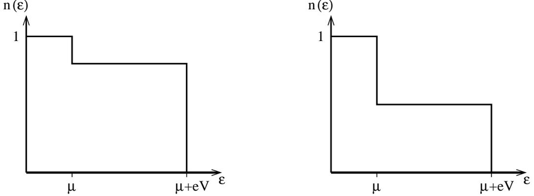
Figure 3.3: The electron distribution function of a wire with negligible energy exchange connected to two reservoirs with electrochemical potentials  $\mu$  and  $\mu + eV$  takes a double-step shape, with the height of the intermediate plateau depending on the position. Left: The distribution function at a position close to the reservoir which is at  $\mu + eV$ . Right: distribution function of the same wire taken at equal distances to the reservoirs.
