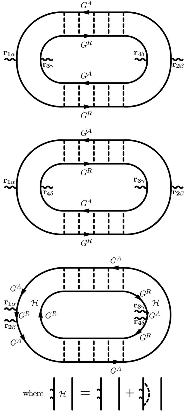
Figure 1.4: Diffuson diagrams contributing to the correlation of conductivity components  $\langle \delta\sigma_{\alpha\beta}(\mathbf{r}_1, \mathbf{r}_2) \delta\sigma_{\gamma\delta}(\mathbf{r}_3, \mathbf{r}_4) \rangle$  resulting in Eq. (1.12). The wiggly lines denote external velocity vertices,  $G^R$  and  $G^A$  the retarded and advanced Green's functions, respectively, and the dashed lines the impurity potential correlator. The impurity ladders (diffusons) are given by Eq. (1.13).
