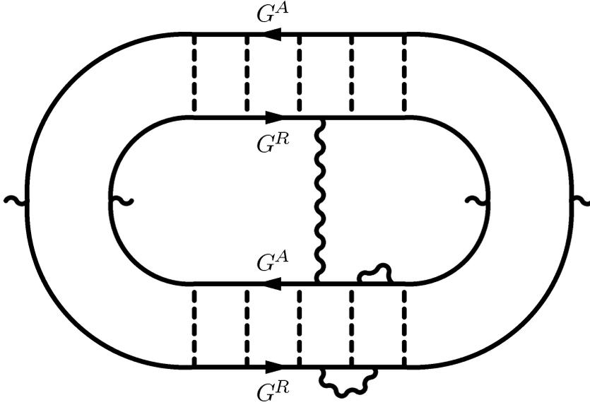
Figure 2.2: Diagrammatic representation of Eq. (2.11). The wiggly lines represent the RPA-screened Coulomb interaction. Since two separate measurements are involved, interaction lines only connect Green's functions corresponding to the same measurement.
