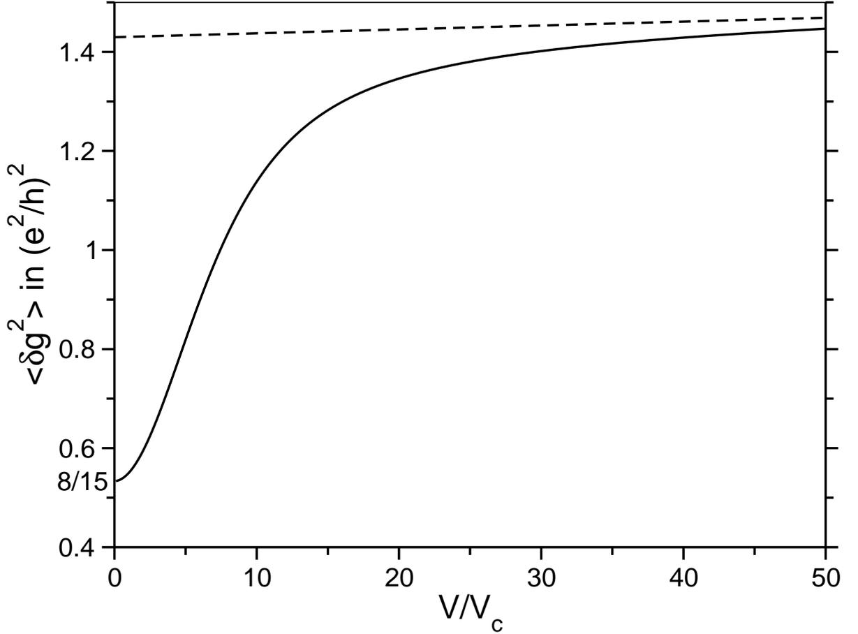
Figure 3.5: Variance of the differential conductance,  $\langle \delta g^2 \rangle$ , as a function of the applied voltage  $V$  normalized to the Thouless energy  $eV_c = D/L^2$ . The dashed line represents the high-voltage asymptotic behaviour,  $\langle \delta g^2 \rangle = 8/15 + c_0 + c_1 V/V_c$  with  $c_0 = 0.8964$  and  $c_1 = 7.785 \cdot 10^{-4}$ , see Eq. (3.54).
