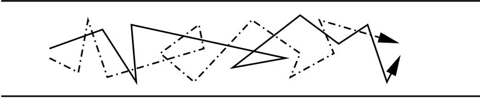
Figure 1.3: Trajectories visiting different impurities interfere with a random sample-specific amplitude. This results in a variance of the conductance over the disorder ensemble which is of order  $e^2/h$ .
