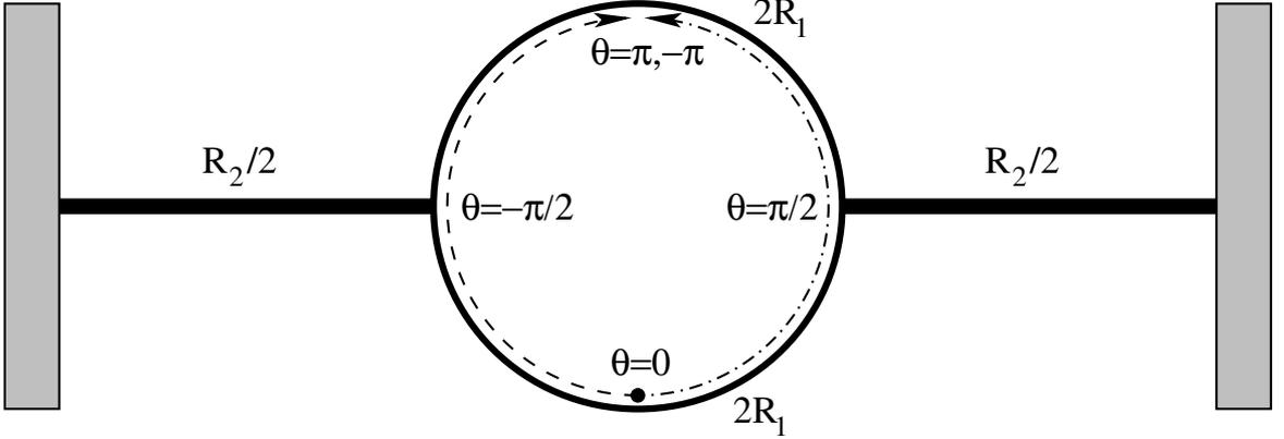
Figure 2.3: The sample geometry and the angular coordinate  $\theta$  suitable to describe the motion along the ring. The paths representing the saddle-point solution derived in Section 2.2.3 are shown. The geometric parameter  $\gamma$  is defined as the ratio of the resistance of the ring without the leads to the resistance of the total sample,  $\gamma = R_1/(R_1 + R_2)$ .
