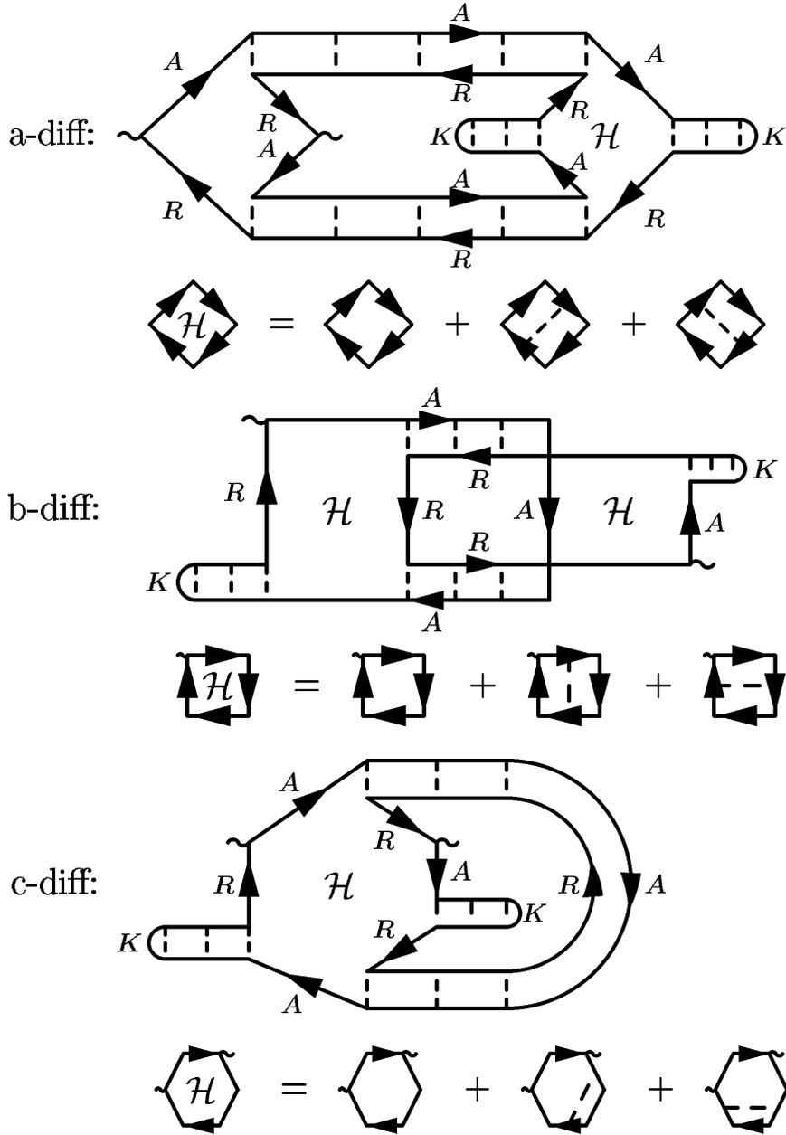
Figure 3.1: The diagrams describing conductance fluctuations are obtained by connecting two diagrams of the type shown in Eq. (3.36) by impurity ladders. With diffuson ladders, these three diagrams can be constructed.  $R$ ,  $A$ , and  $K$  denote the retarded, advanced, and Keldysh Green's function respectively, while the wiggly lines denote the external current vertex. The vertex factors are presented in Appendix C. The three diffuson diagrams sum up to half of Eq. (3.37).
