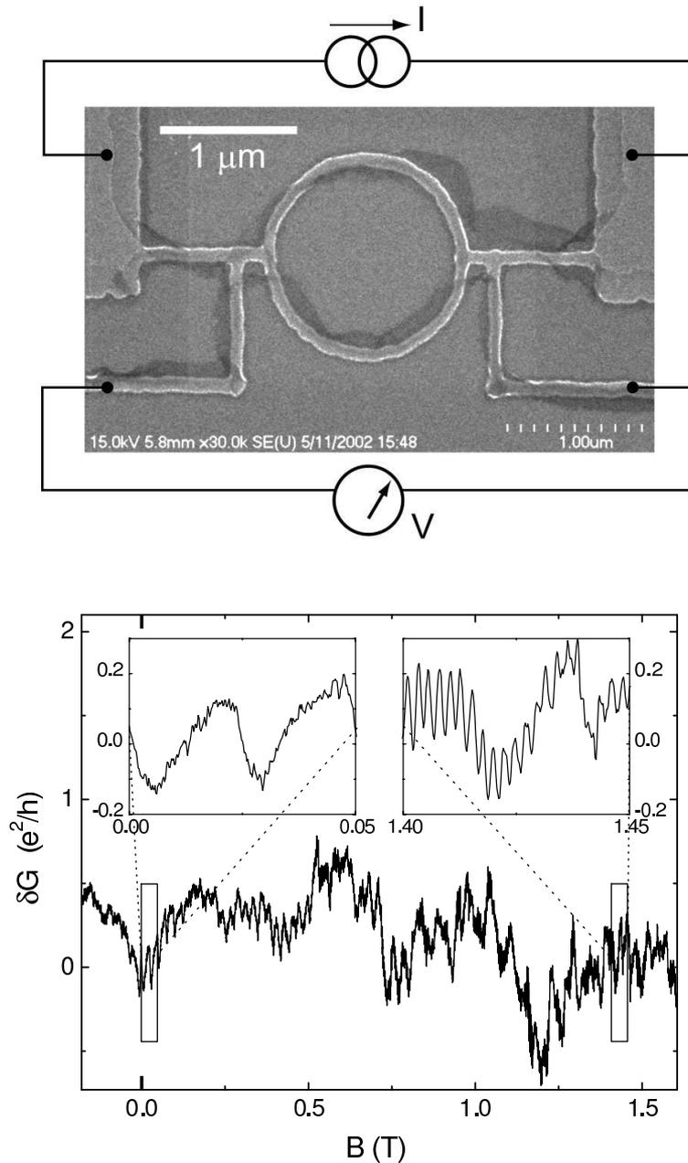
Figure 1.8: Image of an Aharonov-Bohm ring and a magnetofingerprint of this sample, both taken with kind permission from Pierre and Birge [88]. The raw data clearly show Aharonov-Bohm oscillations of the conductance (right inset), superimposed by aperiodic mesoscopic fluctuations on larger field scales. It is also immediately visible from the raw data that at high magnetic fields (right inset) the Aharonov-Bohm oscillations are much stronger than at low magnetic fields (left inset).
