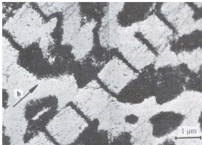
Fig. 2-7 TEM image of dislocation structures (PSBs) in a fatigued Cu crystal [Mughrabi1979].
