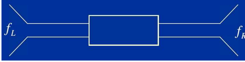
Figure 2.4: Sketch of a scattering region (e.g. a mesoscopic conductor) attached to two electron reservoir leads. The lead electrons are assumed to be in thermal equilibrium and thus their distribution function is given by the Fermi distribution f_L, f_R .
