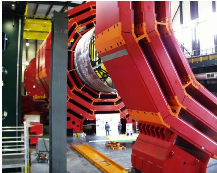
Figure 3.7: The yoke of the CMS detector at an early stage of magnet assembly. [CMS]
