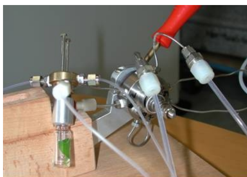
Fig. 10. The head space collected into the vials was transferred into a 10 ml injection loop by flushing the vials with 10 ml of \text{N}_2 . The samples were subsequently injected into the MS.
