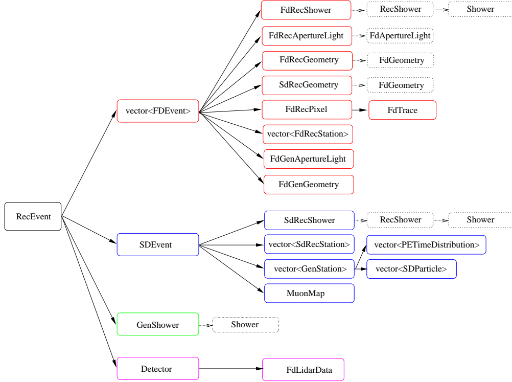
Figure 3.2.11: Data structure of the 'Advanced Data Summary Tree' (ADST, [111]), which has been developed to store all important reconstructed EAS parameters.
