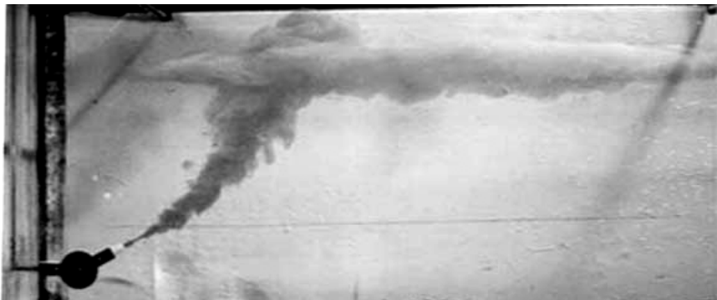
Fig. 4: Laboratory investigation of near-field mixing of submerged discharge into a stratified water body. The initial buoyant jet motion is followed by trapping and internal spreading at the terminal level.
