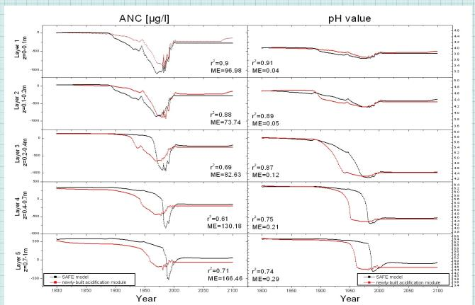
Shown is a test simulation at the Solling site for ANC (acid neutralization capacity) on the left, and the pH value on the right hand side. The newly-built acidification module shows good agreement to the SAFE model results in the uppermost two layers. With increasing depth, the simulation results diverge. This can have several reasons: differently simulated water percolation, which mainly influences soil moisture, or plant uptake of base cations.
