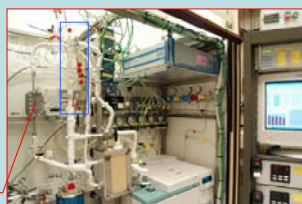
Figure 3. Lab equipment with control unit and gas analyzers. On the left side one can see the micro-reactor. Right of it the tubular fixed bed reactor is to be seen (blue frame).
