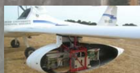
AEROSOL SIZE DISTR. 5 nm – 20 μm (GRIMM) + > 10 nm (TSI 3010)
