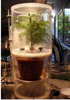
Fig. 2. Spruce sapling in the twin cuvette for separate measurements of above- and belowground compartment.
