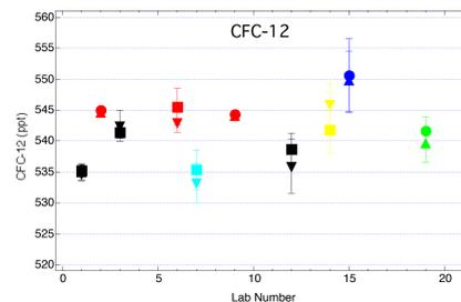
Ten labs reported CFC-12 on six scales. Scale differences of 2-3% are evident.
