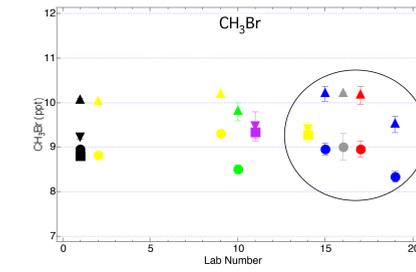
Most labs observed a 0.2 or 1.2 ppt difference between cylinders filled in summer and winter. There is also good agreement among CH<sub>3</sub>Br scales even though the long-term storage of CH<sub>3</sub>Br in cylinders can be problematic.
