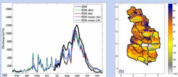
(a) Routed vs. measured discharge [m<sup>3</sup>/s] for Nawuni, outlet of complete basin (2004) using IDW and EDK with several external drifts as spatial interpolation methods for precipitation; (b) Spatial distribution of differences of total runoff resulting from the applied interpolation methods EDK (long-term mean annual rain) and IDW for areal precipitation
