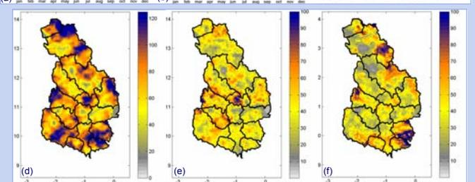
Spatially averaged daily range (grey) and mean (black) for precipitation (a), actual evapotranspiration (b), and discharge at Nawuni, outlet of complete basin (c) using all turning band simulation results; corresponding spatial distributions of standard deviation (d) to (f) [mm]
