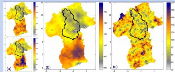
(a) Two random realizations, (b) mean, and (c) standard deviation of turning band simulations for annual precipitation [mm] for 2004
