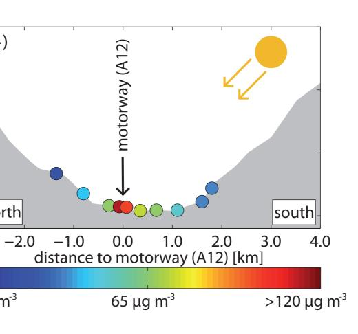
of NO<sub>2</sub> in the valley cross section (Fig.24/25). Higher concentrations were found at the sunny slope each period. This is mainly due to local slope winds and the proximity to motorway. Maximum values were measured at the valley bottom and near the motorway.
