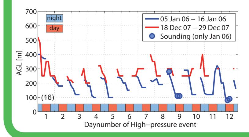
Subjective analysis of the mixing layer height from ceilometer backscatter intensities during high pressure events illustrates the daily variation of them. Typically, the MLH is lower in the evening/ night and higher from noon to afternoon (Fig.16). Generally, the mixing layer 2005/06 was lower than in 2007/08.
