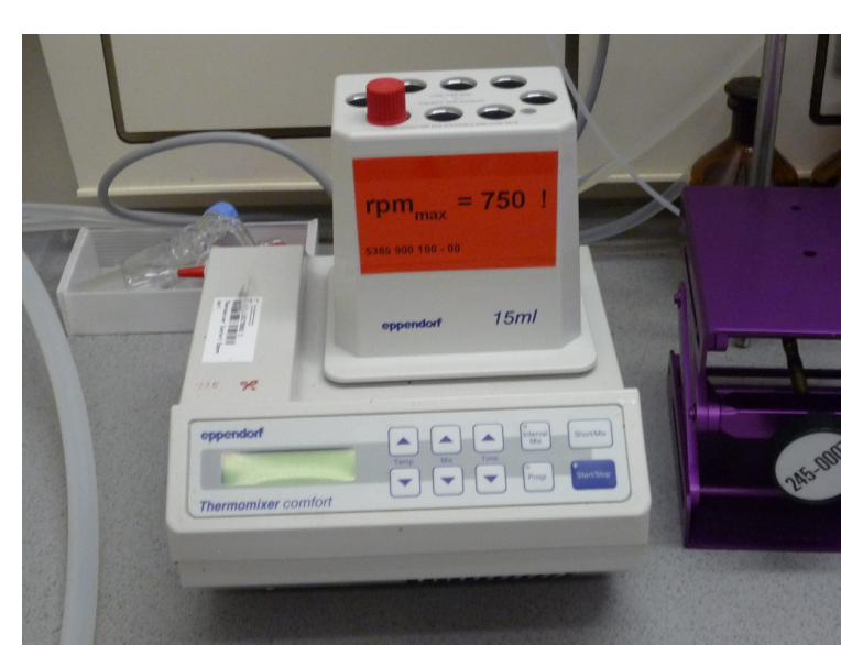
Fot. 2. Agitation in the thermomixer
