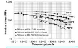
Experimental stress-rupture curves in comparison to literature
