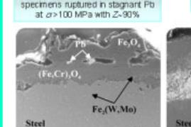
Pb in the outer oxide layer
