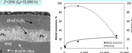
Exposure time effect on metal recession and necking
