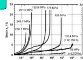
The strain-time curves in range of 75-325 MPa
