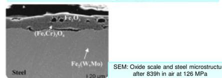
SEM: Oxide scale and steel microstructure after 839h in air at 126 MPa
