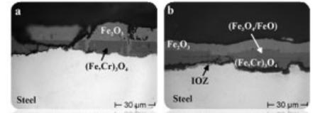
SEM: Oxide scale formed at the beginning of the necking region (a) and far from the fracture surface (b)
