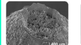
Typical ductile fracture of the specimens ruptured in stagnant Pb at  $\sigma > 100$  MPa with Z=90%
