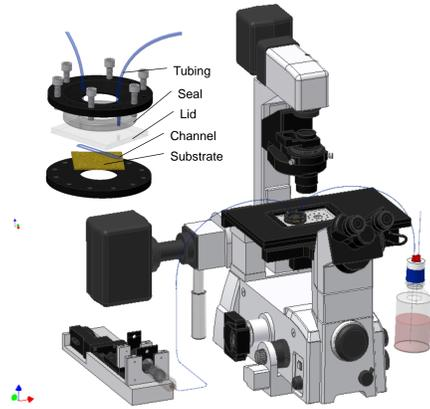
The setup: incubation microscope with syringe pump, microchannel and liquid reservoir.
