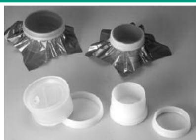
We use 40 mm Disposable Closed X-Ray Cells from SPEX SamplePrep. The cells consist of a polyethylene snap-ring and cup with snap-post vent and reservoir. After settling the biofouling organism on a 8 µm Kapton film, the reservoirs are filled with the medium or artificial sea water and the Kapton film is placed on top of the cell. Afterwards the cells are sealed with the snap-ring. Now the water-tight sample can be placed in a sample holder and the XRF microprobe scans can be performed.
