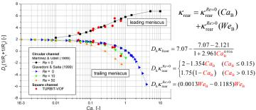
> Relating the unknown bubble velocity to the given total superficial velocity
