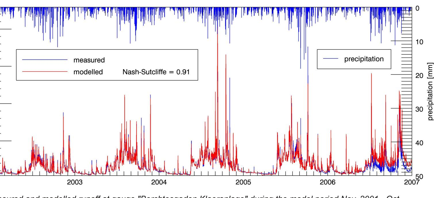
Measured and modelled runoff at gauge "Berchtesgaden Klaeranlage" during the model period Nov. 2001 - Oct. 2007 in m<sup>3</sup>/s (routed runoff rates replaced by observed discharges)
