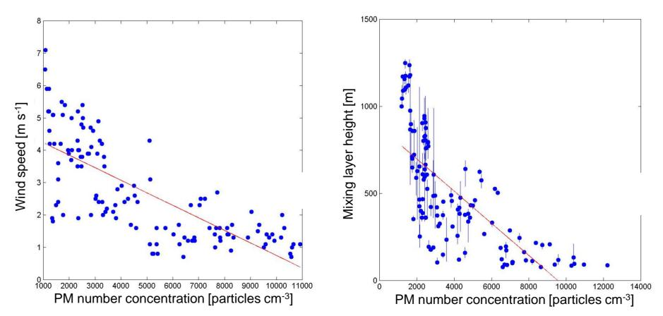
Comparison of the hourly-mean values of PM number concentrations in the size range 100 – 500 nm with hourly-mean mixing layer height (MLH) values (left) and wind speeds (right) during winter 2008. As an example a linear regression function is given.
