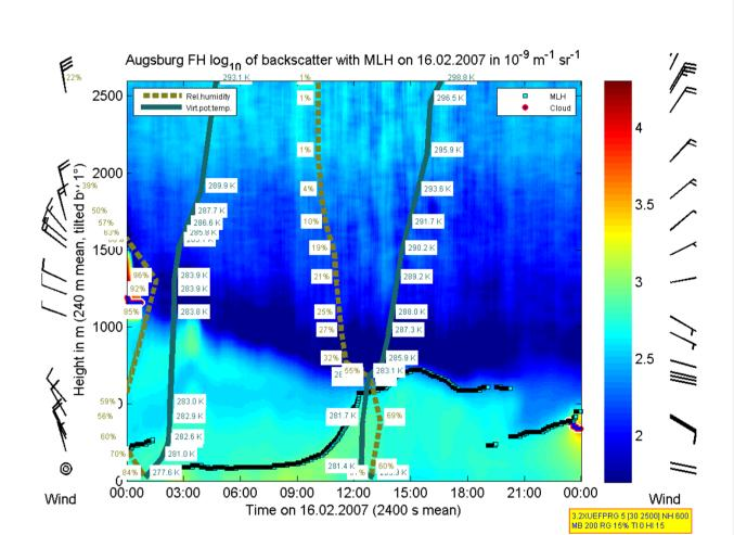
Measurement results of ceilometer Vaisala CL31 to observe the vertical aerosol distribution together with radiosonde data (wind vector, relative humidity and potential virtual temperature) from the meteorological observatory Oberschleißheim on 16 February 2007 (left) and 16 February 2008 (right). The time is given as local time. The backscatter intensity is presented in different colours (see right part of the figure). The mixing layer height (MLH) is given by blue squares.
