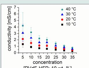
Conductivity of MPPyrr-TFSA based gel electrolytes as a function of the PVdF-HFP concentration at different temperatures.  $c$  (LiTFSAs) = 0.5 mol/kg
