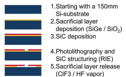
Fig. 2 Basic process flow for the fabrication of the test structures
