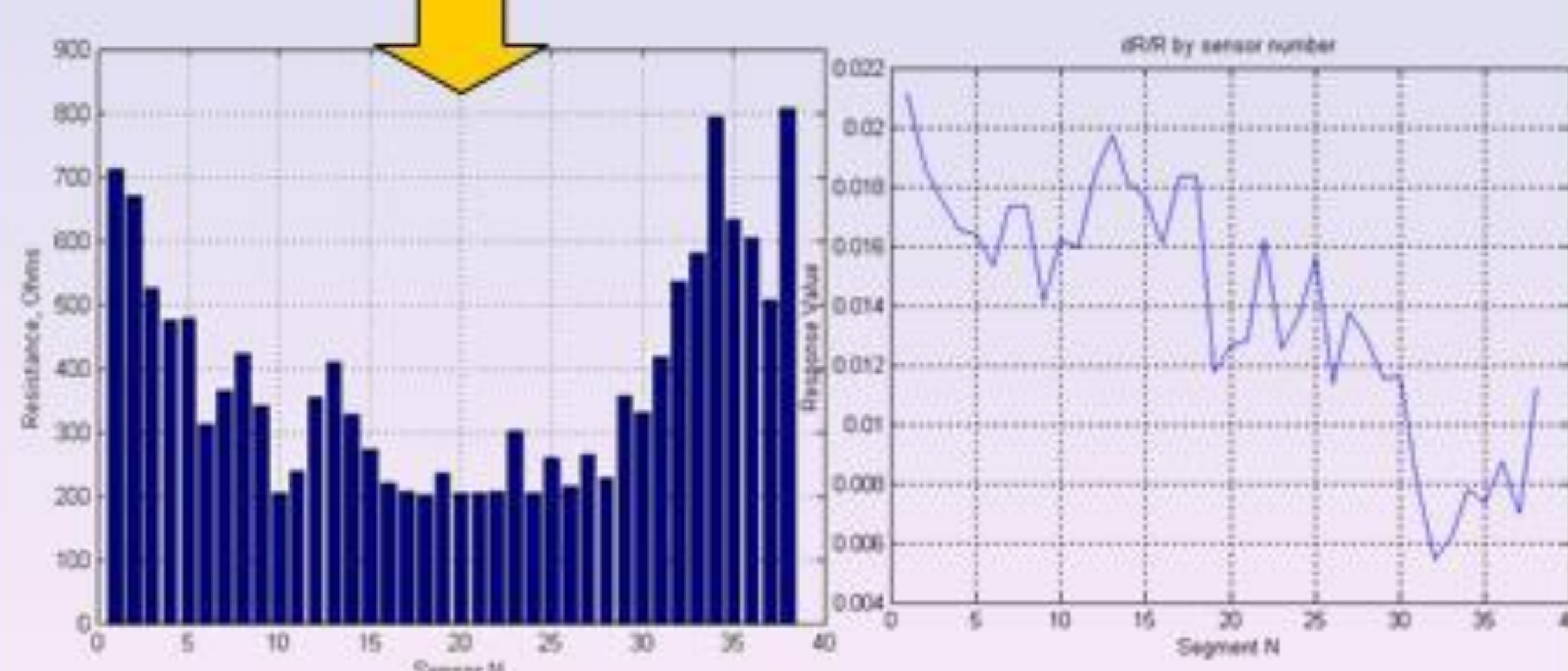
Fig. 2: The fabricated chip prototype and measured distribution of graphene segment resistance over the array
