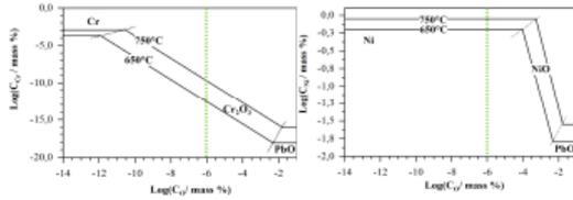
Fig.1 Concentration of Ni and Cr dissolved in Pb at 650/750 °C, green line shows the experimental oxygen concentration in the liquid lead
