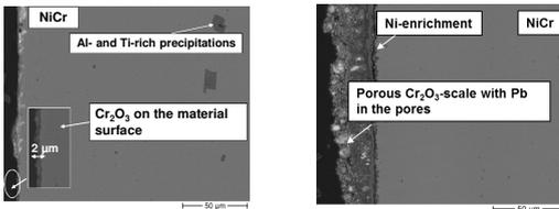
Fig.4 SEM/EDX Analysis of the cross-section of Ni48Cr alloy
