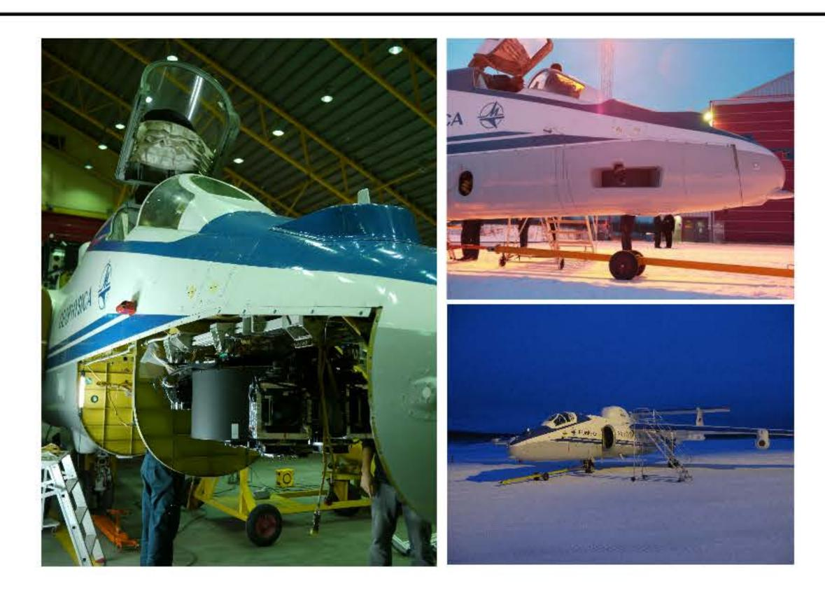
The M-55 Geophysica carrier aircraft. The pictures to the left and the upper right show GLORIA deployed in the plane's forward bellypod. The aft bellypod (visible in the left image) is reserved for the MARSHALS sounder which was also mounted for ESSenCe.
